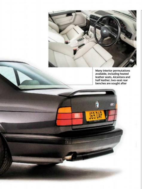
**Interiors** are time-consuming to put right if scruffy, but not too costly if you shop around specialist breakers. If originality is important, check the spec - some have been updated with later trim. Check under the passenger seat for damp near the underseat modules, make sure the sides of the front seat backrests haven't collapsed (an easy DIY fix if you're happy dismantling a seat), and check the door cards for delamination. Ensure sunroof and aircon work.
