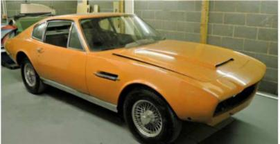
This very subtle crease is easy to miss unless you know what to look for. Every DBS should have a straight contour that starts behind the front wheel and continues at tyre-top height through the door and rear wing. It would prove to be a key challenge later in the bodywork repairs, but first the DBS needed blasting.
