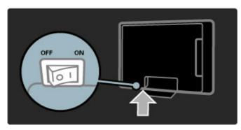
If the red indicator light is off, switch on the  $\mathsf{TV}$  with the power switch.
