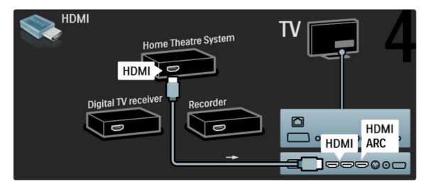
If you do not use the HDMI-ARC connection on the TV and the device, add a digital audio cable (cinch coaxial).
