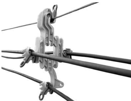
The ECL-15 cable spacer can be attached to the messenger wire with a snap tie.
