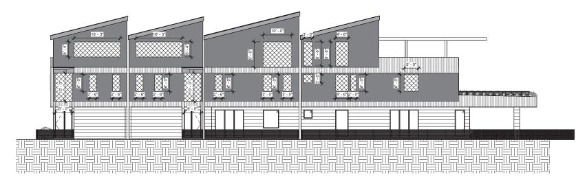
SOUTH ELEVATION OPENING DIAGRAM 3/32" = 1'-0"
