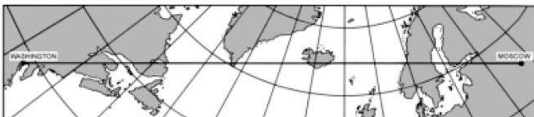
Figure 309d. An oblique Mercator map based upon a cylinder tangent along the great circle through Washington and Moscow. The map includes an area 500 miles on each side of the great circle. The limits of this map are indicated on the Mercator map of Figure 309c
