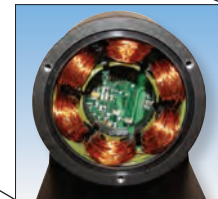
Cut-away view showing integrated drive on 74215-series and 74445-series pumps.
