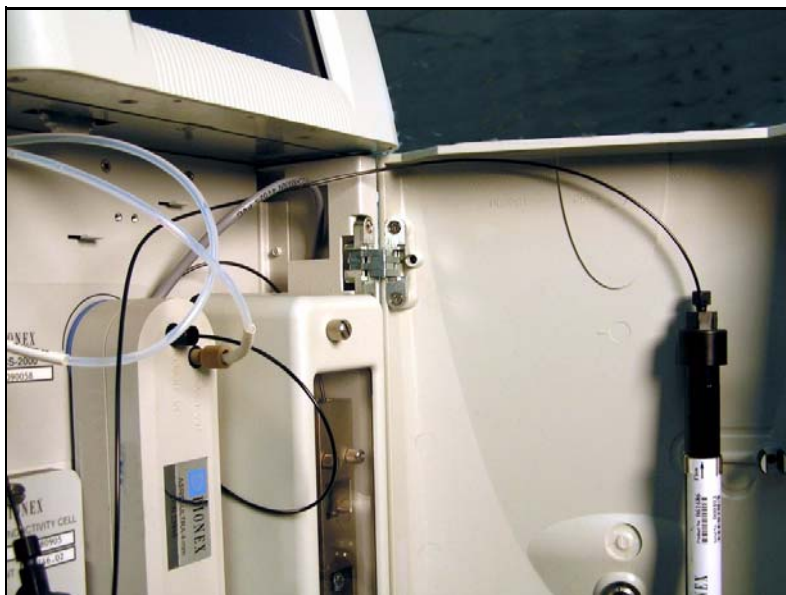
Figure 81. Mixer Outlet Routed to the Back of the Component Panel
