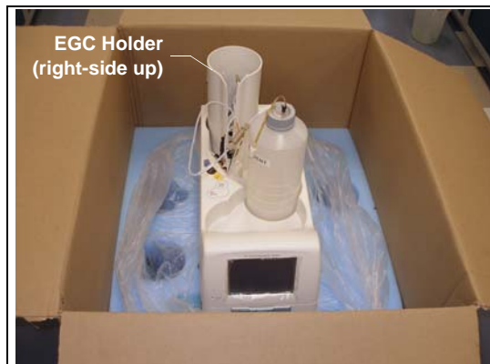
Figure 3. ICS-2100 After Installing Eluent Bottle and EGC Holder
