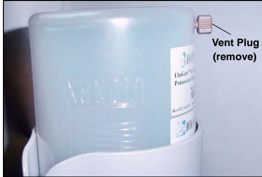
Figure 90. EluGen Cartridge Vent Plug
