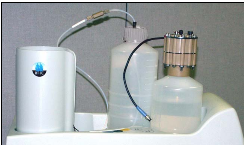
Figure 85. EluGen Cartridge in Service Area
