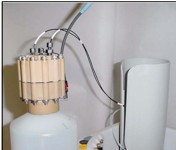
Figure 52. EGC Inlet and Outlet Connections
