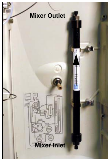
Figure 95. EGC CO 3 Mixer Installed on the ICS-2100 Door
