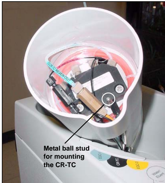
Figure 38. Cartridge Holder (Tilted to View the Bottom)
