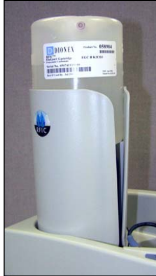
Figure 87. EluGen Cartridge Installed in the Holder
