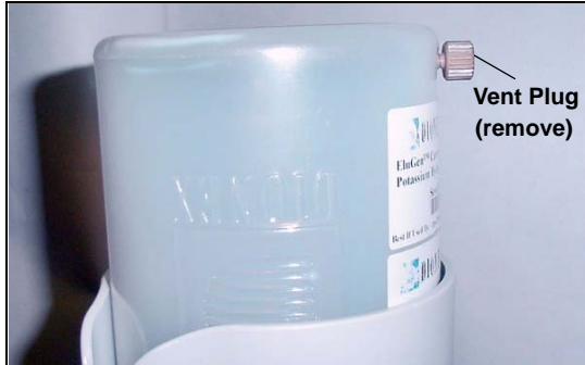
Figure 49. EluGen Cartridge Vent Plug
