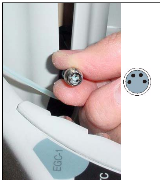
Figure 48. Connecting the EluGen Cartridge Cable
