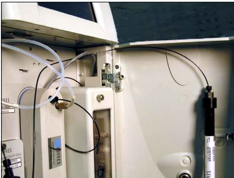
Figure 98. Mixer Outlet Routed to the Back of the Component Panel
