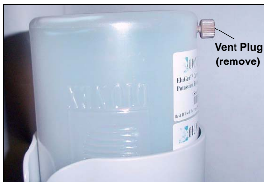
Figure 65. EluGen Cartridge Vent Plug
