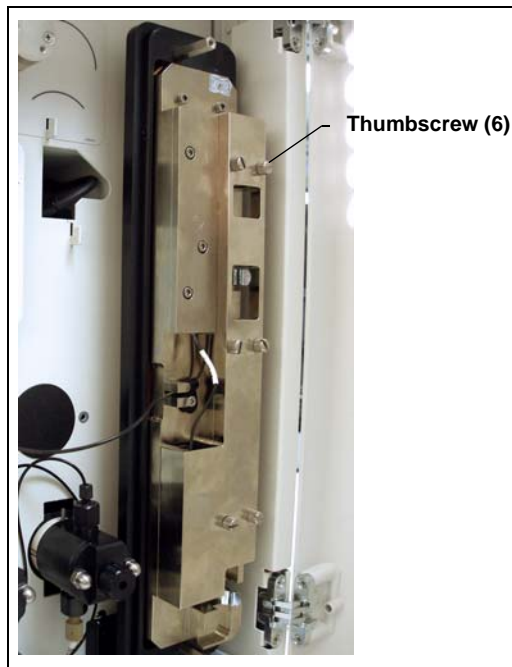
Figure 28. Column Heater with Cover Removed
