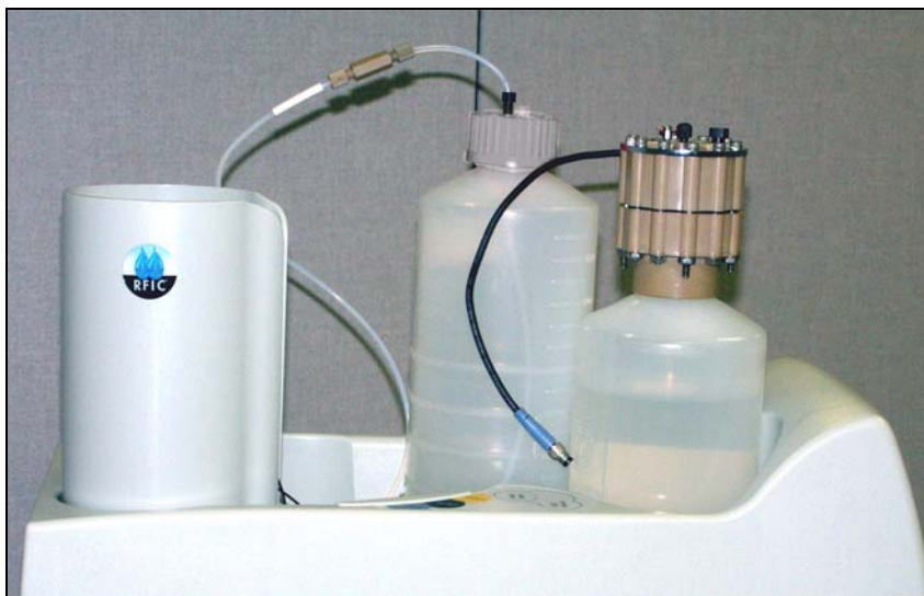
Figure 44. EluGen Cartridge in Service Area
