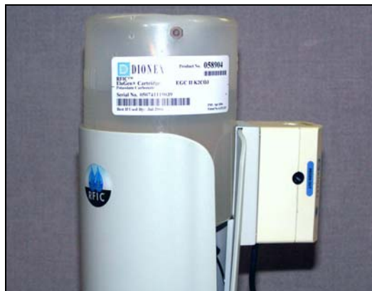
Figure 68. EPM and Mounting Bracket Installed on EGC Holder
