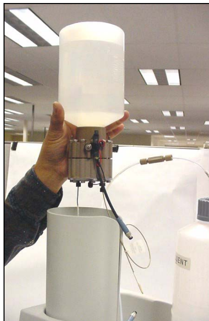
Figure 47. Installing the EluGen Cartridge in the Holder
