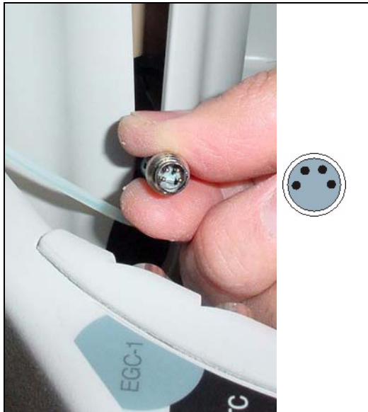
Figure 88. Connecting the EluGen Cartridge Cable
