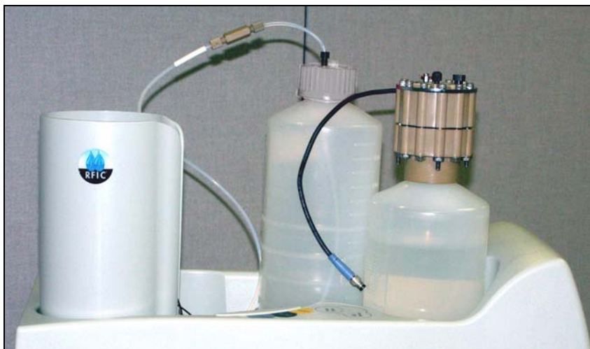
Figure 61. EluGen Cartridge in Service Area
