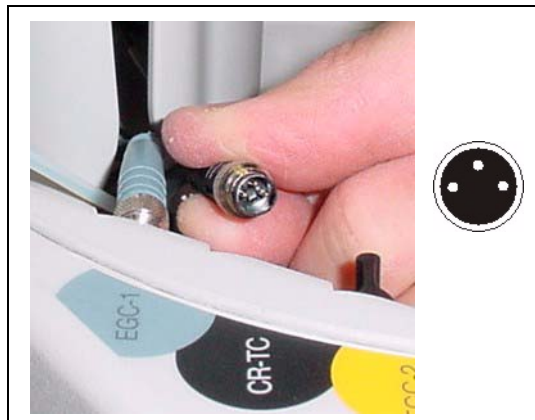
Figure 54. Connecting the CR-TC Cable
