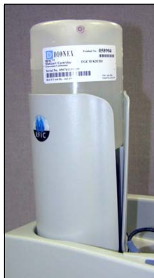
Figure 63. EluGen Cartridge Installed in the Holder
