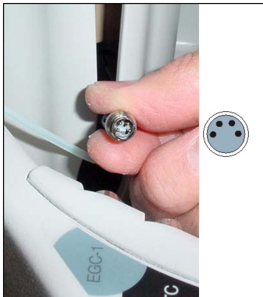
Figure 64. Connecting the EluGen Cartridge Cable
