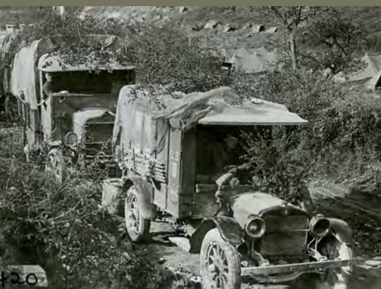
A GMC Ambulance is leading an AEC Y Type as a rather heavily camouflaged sanitary train is described as being on the move
