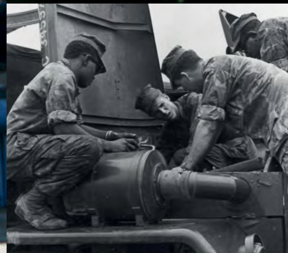
Members of 7th Motor Transport Battalion mull over a problem with the multi-fuel/diesel engine of an M54 series truck. The photograph was taken some time in 1969 (SERGEANT CURTIS / 26393928)
