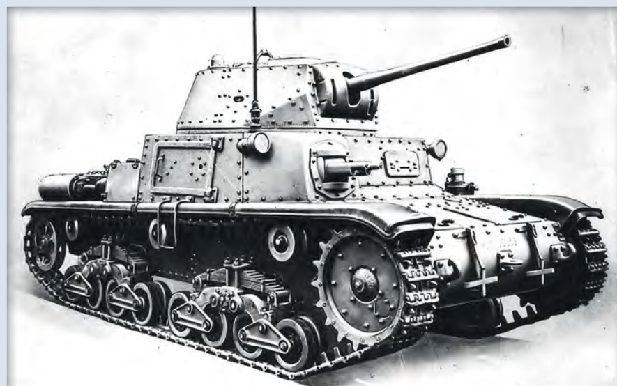
An M15/42 from the other side, showing the new location of the hull escape door
