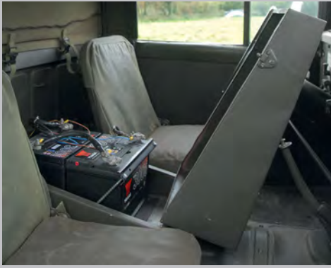
The large battery box between the crew seats contains two very beefy batteries to accommodate the 100amp charging system
