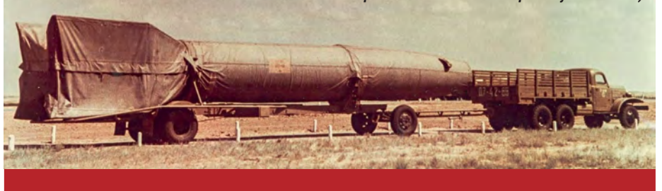
BELOW: An R-2 rocket being towed by a 6x6 ZiS-151 truck at the Kapustin Yar polygon. The standard production ZiS-151 dates the photograph as the very early 1950s rather than late 1940s (early production ZiS-151s produced from 1948 had a partially wooden cab)
