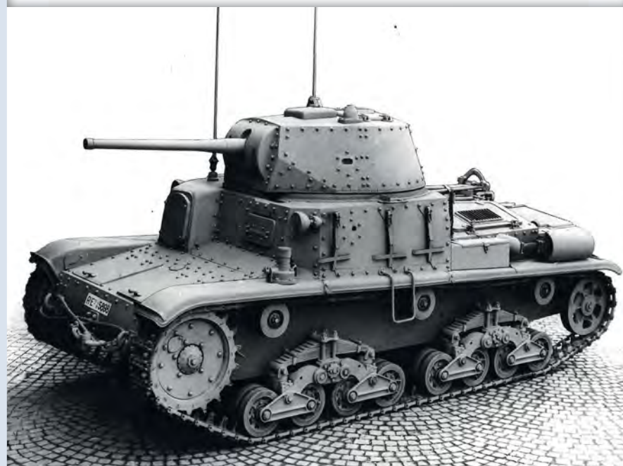
ABOVE: Despite a more powerful engine and better gun the M15/42 looks a lot like its predecessors BELOW: A P26/40 viewed from the front, sloped armour makes it look impressive but it wasn't very thick by infantry tank standards and the method of construction was going out of favour
