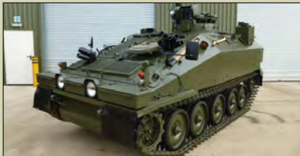
Spartan CVRT Dieselised APC , Fitted Cummins BTA 5.9lt Turbo diesel engine, Engine: power 195 hp, David Brown TN15d Epicyclic Semi-Automatic Gearbox with Neutral turn capability, Max road speed 72 km/h, Range 750 km, Manoeuvrability, Gradient 60%, Side slope 35%, Vertical step 0.5 m, Trench 2m, Fording 1m etc, Ex condition, ..... Price from £19,995 (1 Available)
