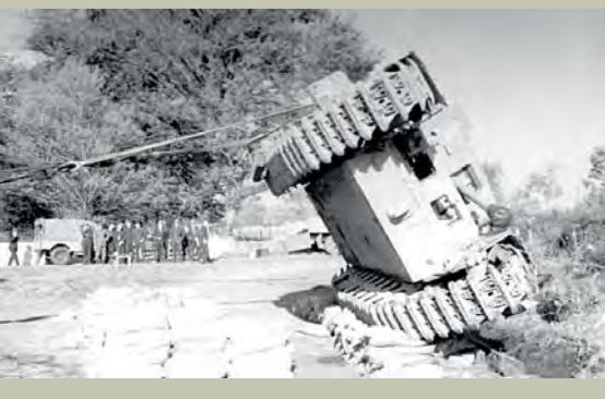
BELOW: The overturned tank is pulled back onto its tracks. The sandbags have been placed to protect the road surface and cushion the impact of the fall
