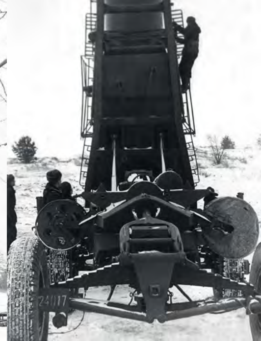
ABOVE LEFT: The Soviet successor to the V-2 in firing position on the Russian steppe, without protection from the elements ABOVE RIGHT: The 8U24 transporter-erector trailer for the R-1 was a basic assembly intended for limited distance travel only. Note the conventional truck-type leaf-spring for shock absorption
