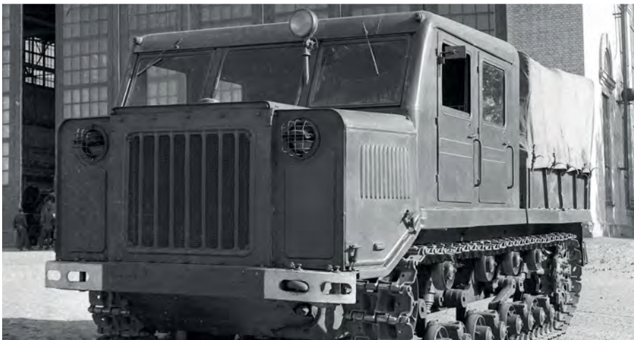
ABOVE: The AT-S medium artillery tractor was developed to replace the wartime Ya-12 and post-war M-2. The vehicle could accommodate a six-man gun or rocket crew in addition to the driver BELOW: A side view of the same vehicle, with its twin-cab and rear cargo area. The tracked AT-S and AT-T tractors and the wheeled 6x6 ZiS-151 were all used to move R-1 and R-2 rockets on their transport-erector trailers
