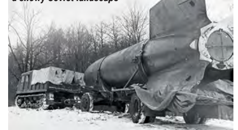
An AT-S medium tracked artillery tractor towing an R-1 (8Zh38) rocket across a snowy Soviet landscape
