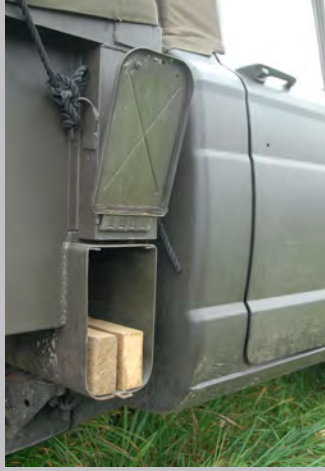
The stowage which sits behind the cab on each side is a military addition
