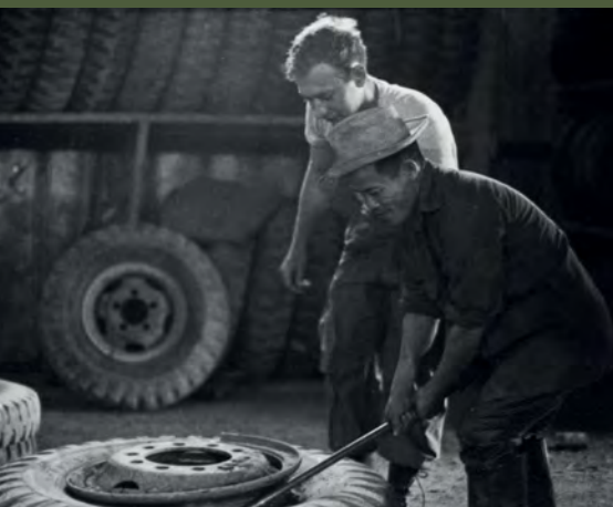
The 1st Force Service Regiment deployed a large number of trucks to deliver such as food, fuel, water and ammunition to marines deployed in the field. Maintenance personnel had to deal with an average of 50 punctured tyres every day. Here we see Corporal Raymond T Bruton on December 23, 1968, training a Vietnamese civilian employee on how to deal with a punctured tyre (CORPORAL JOHN S KRILL / 26393781)
