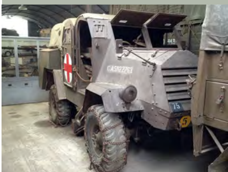
The impressive bulk of the 1944 Chevrolet C15TA weighs in at four-and-a-half tons. They were used as armoured personnel carriers or ambulances
