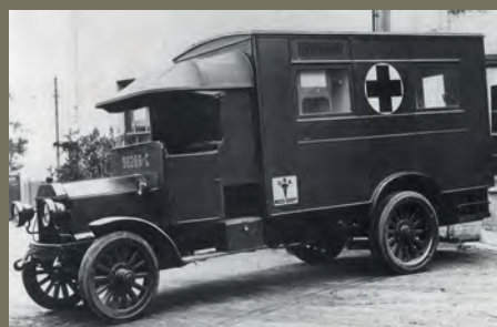
An unusual sight is this American-built Peerless TC4 truck which has been fitted with a medical department laboratory body in Britain
