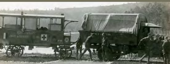
This Pierce Arrow truck is towing a mobile laundry trailer, vital equipment to help prevent the spread of disease within the mobile hospital
