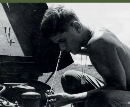
Private First Class George Kreiner, a member of C Company, 9th Motor Transport Battalion, checks the oil level of an M series truck (26403691)
