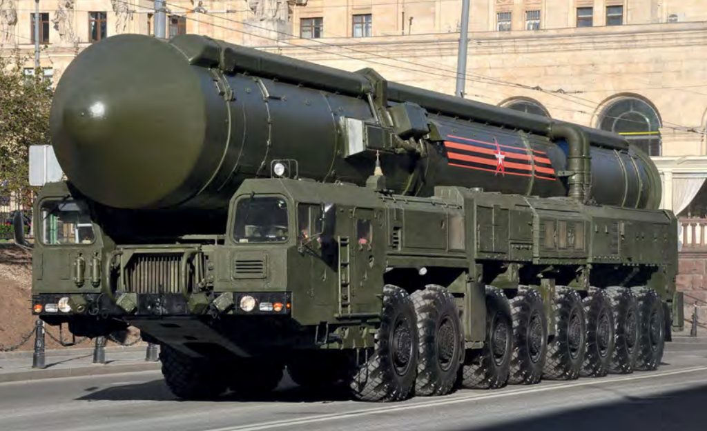
ABOVE: The RS-24, 11,000km range intercontinental rocket is mounted on the eight-axle MZKT-79221 chassis. The system is the result of a half-century of further technological development into road mobile strategic rockets, which all started with the V-2 in 1944
