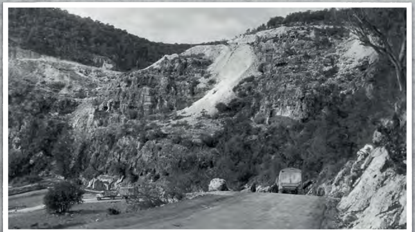
For the passage through the mountainous terrain of the Wadi El-Kouf, the 6x4 Fordsons have been unhooked from the mobile darkrooms and replaced by 4x2 lorries: a Dennis AM 30/40 cwt (as seen here) and a Chevrolet. A likely reason for this is that the 6x4s provided better traction in the sands of the desert, and that the 4x2s will provide better braking in the mountains. The Dennis was built specially for the Air Ministry, and has a two-speed transfer box and a vacuum brake pipe to the rear allowing it to work a trailer's brakes. The Chevrolet may not have the vacuum brake pipe, but unlike the Fordsons which have mechanical brakes, it has powerful servo-assisted hydraulic brakes
