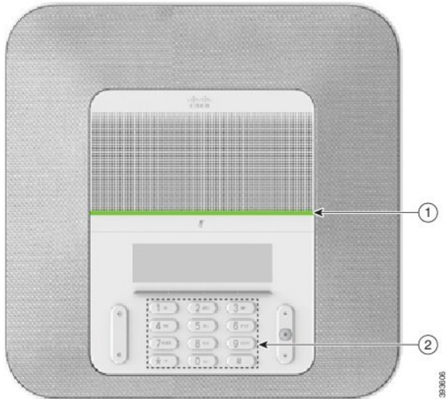
Figure 17: Mobility-Impaired Accessibility Features
