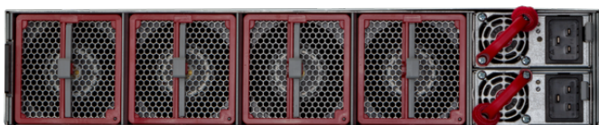
Arista 7280R3 2RU Rear View: Front to Rear airflow (red)
