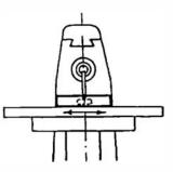
Fig. 67. Checking Parallelism of T-slot with the Table]Movement
