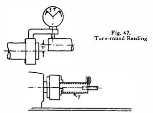
Fig. 48. Tubular Holder for Dial Gauge
