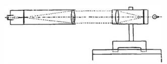
Fig. 10. Diagram illustrating the Principle of Testing by means of Target and Telescope
