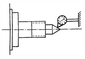
Fig. 40A. Checking the Centre
