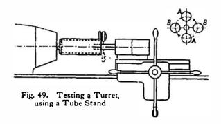
(a) The swing-over or turn-round method. This has been shown and discussed in Figs. 1A, 19 and 47. The dial gauge must be of the required accuracy and the mandrel of the necessary size and stiffness. Readings are taken at 180° positions in the horizontal and vertical planes, and, as mentioned above, the alignment error is equal to half the difference between two diametrically opposite readings.
