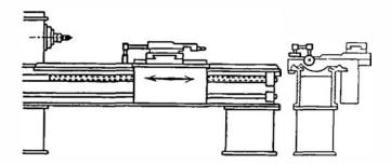
Fig. 37. Acceptance Test for Guideways
