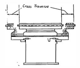
Fig. 28. Table that is Shorter than its Slideway by an amount equal to the Cross-traverse of the Table
