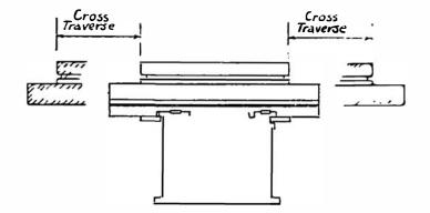
Fig. 29. Table with Length equal to that of the Slideway
