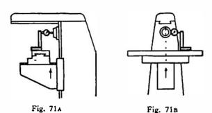
Fig. 71A and 71B. Perpendicularity between Table Surface and Columnway for the Knee
