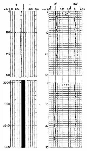
Fig. 22 (Left) Test chart for an accurate lead screw.
