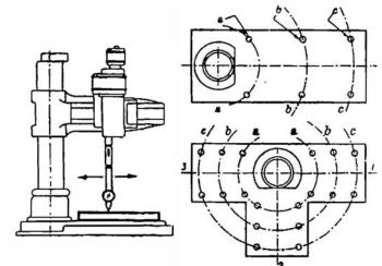
Fig. 85A. Parallellam of Drilling-head Slideways and Base
