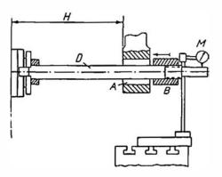
Fig. 53. Slip-bushing Method
