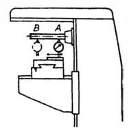
Fig. 63. Parallelism between the Surface of the Table and the Spindle Axis
