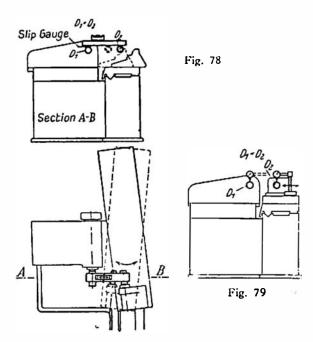
If the grinding-wheel spindle has a cylindrical portion, this may be used instead of test mandrel  $D_1$ . In this case the difference between the diameter of test mandrel  $D_2$ and that of the spindle cylinder must be compensated by block gauges.
