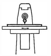
Fig. 64. Parallelism between the Table Surface and the Direction of the Longitudinal Table Movement
