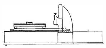
Fig. 68. Testing Inclination of Bed with Parallels, Straight-edge and Spirit-level
