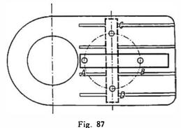
after the latter has been levelled. The dial gauge is fixed to the spindle, the dial-gauge plunger touching the straightedge. The drilling head is traversed over the whole length of the radial arm. The reading of the dial gauge must not vary by more than 0.2 millimetre/1,000 millimetres (0.0025
