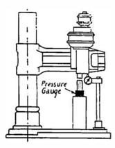
Fig. 91. Testing Vertical Thrust on Drilling Machine
