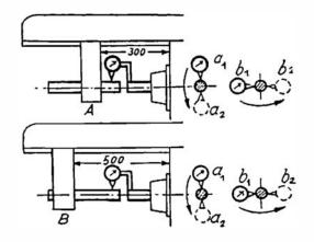
Fig. 52. Checking Spindle Alignment
