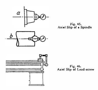
which rests in the centre bore (Fig. 45b). The first method (Fig. 45a) is often used when axial slip of the spindle is measured, the second method (Fig. 45b and Fig. 46) is employed for testing the axial slip of lead-screws.
