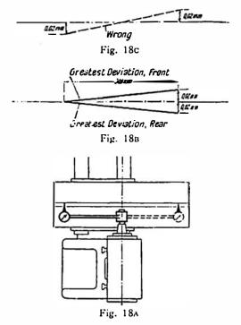
Figs. 18A, 18B and 18C. Tolerances in Measuring by the Turn-round Method
