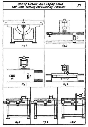
It is evident that the high degree of accuracy which is usual in metal working is not obtainable, nor called for, in woodworking. Hence acceptance tests for woodworking machines can be comparatively simple and provide for fairly coarse tolerances, partly because woodworking machines are much simpler in design than those for metal working.
