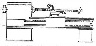
Fig. 4. Mandrel running out of Truth must be set to Mean Position before Testing for Parallelism with the Bed
