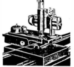
Fig. 8. Method of Testing by means of a Tau Wire and Measuring Microscope
