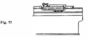
gauge plunger touching the test mandrel (for measurement in the vertical plane). The table is moved longitudinally and readings are taken. The tailstock centre must be higher than the headstock centre. Measurement in the horizontal plane is not necessary, as alignment in this plane is adjustable.
