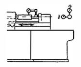
Fig. 75. Testing Parallelism between Grinding-wheel Spindle and Table Movement
