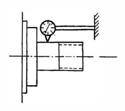
Fig. 40D. Checking a Cylinder
