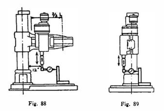
readings can only be taken at the 0° and 180° positions (A and B). The 90° and 270° measurements, (C and D) must be taken after the straight-edge has been turned 90°. This method is more cumbersome and waviness or irregularities of the base plate surface are covered up.
