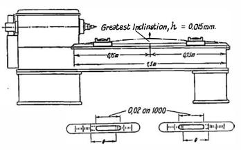
Fig. 13. Unilateral Tolerances in Spirit-level Measurements
