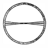
Care must be taken, however, that the wire is free from kinks. The wire diameter should be as small as possible, in any case not more than 0.1 millimetre (0.004 inch). Long beds up to 20 metres (65 feet) and more can be tested without the need for special precautions. For greater lengths it may be necessary to damp the vibrations of the wire by suitable means, for example, by attaching small paper tags which are suspended in oil.
