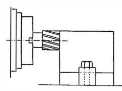
Fig. 90B. Performance Test on Milling Machine— Face Milling
