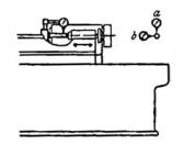
Fig. 74. Parallelism between Tailstock Sleeve and Direction of Table Traverse
