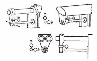
Fig. 69. Parallelism between Overarm and Spindle Axis
