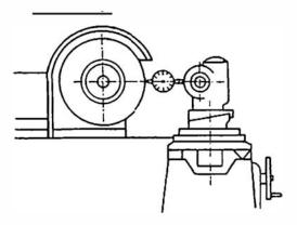
Fig. 90c. Fine In-feed Test
