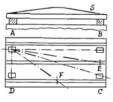
Fig. 36. Checking Flatness of Table
