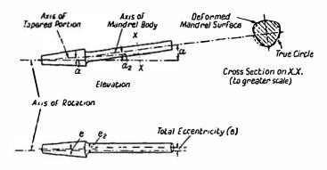
Plan Fig. 41. Sources of Error in Rotating Mandrols
