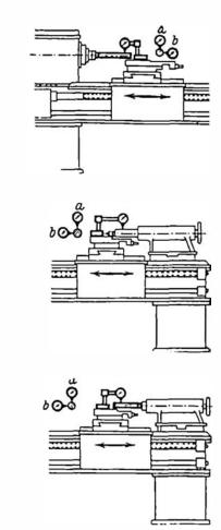
(A) IN THE CASE OF THE CENTRE LATHE, parallelism has to be checked:
