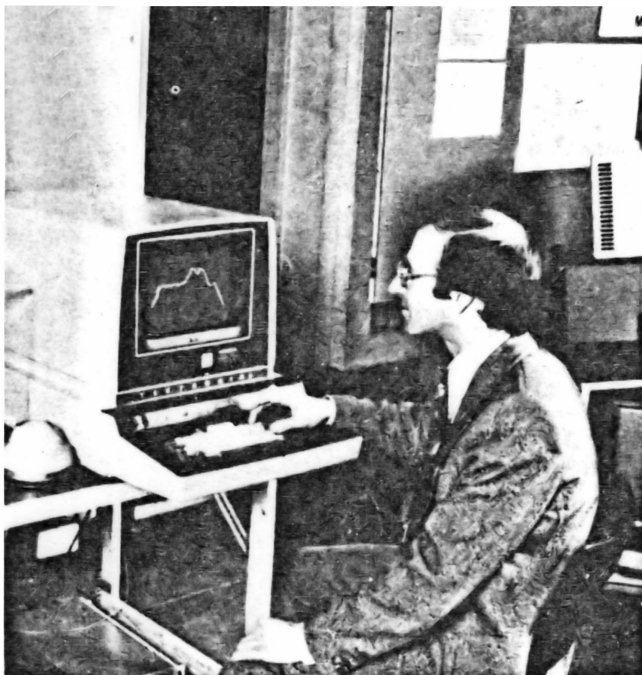
Fig. 18. Computer-aided design of a loudspeaker cone using a visual display.
