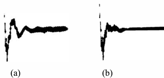
Fig. 10. Transients obtained by acoustic measurements: (a) closed box w/electric damping (b) acoustically damped box w/electric damping
