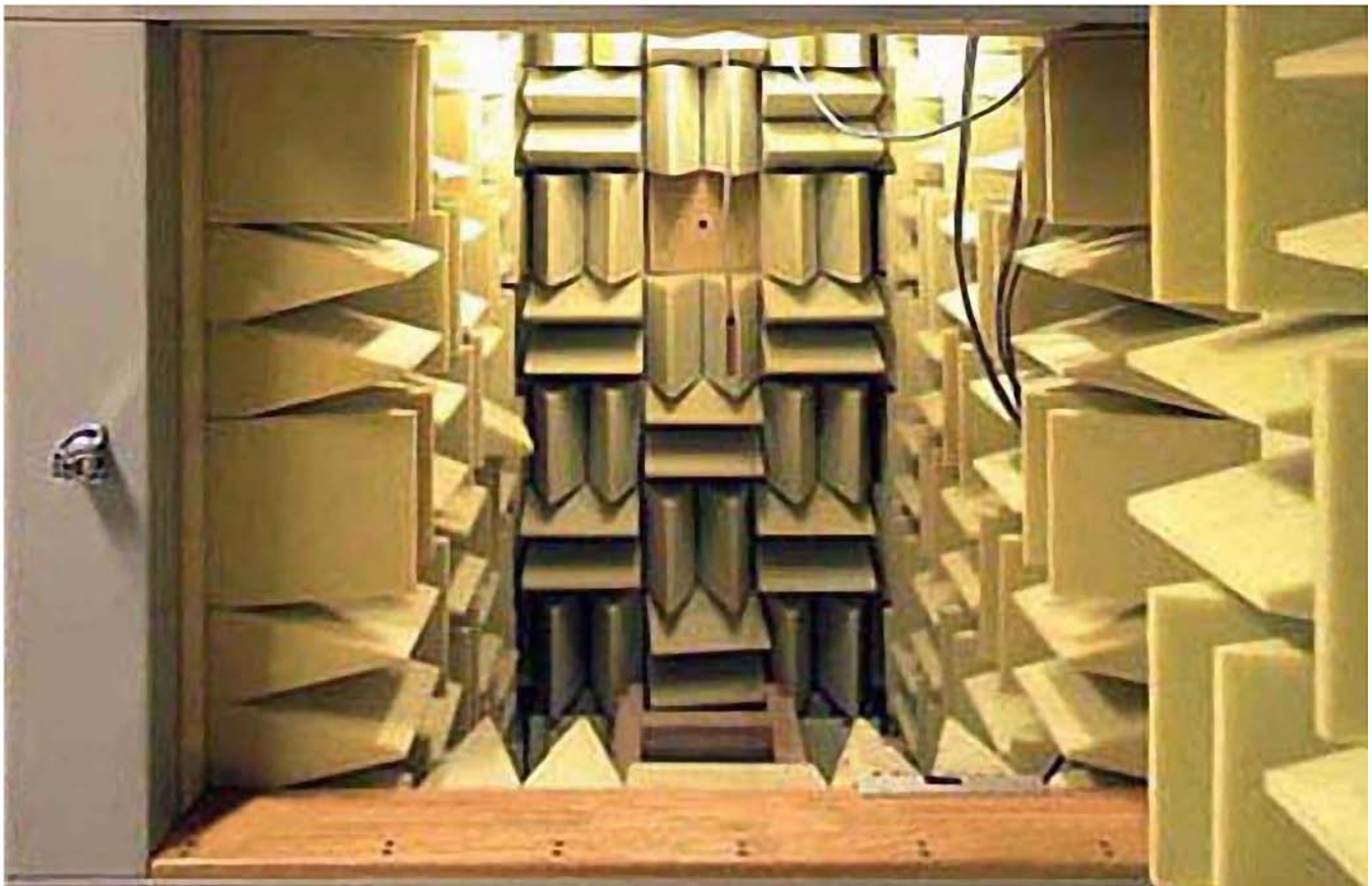
FIG 8.1 Tweeter frequency response measurement in the production anechoic chamber. All drive units used in PR Two production are subjected to rigorous inspection and measurement.
