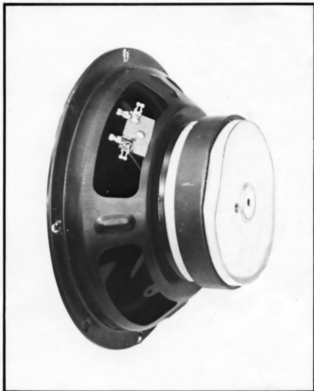
FIG 3.1 The 200mm bass unit showing the large magnet structure. Note the vent holes in the back plate and in the pole piece. These vent a cavity in the magnet structure and prevent pressure build up from expelling the FERROFLUID.
