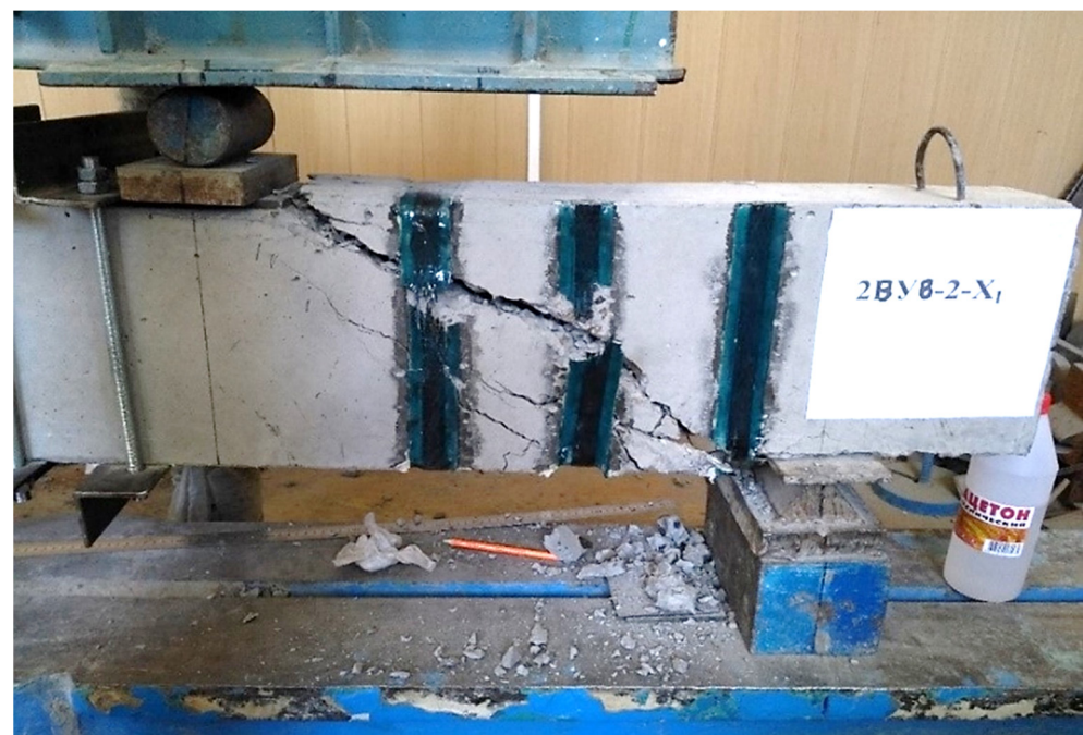
Figure 7. The nature of the collapse of the prototype No. 40, reinforced with U-shaped stirrups during the cut 2.5 h_0 .
