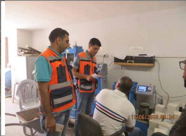
14. Follow up breaking concrete cubes at Hijjawi lab.
