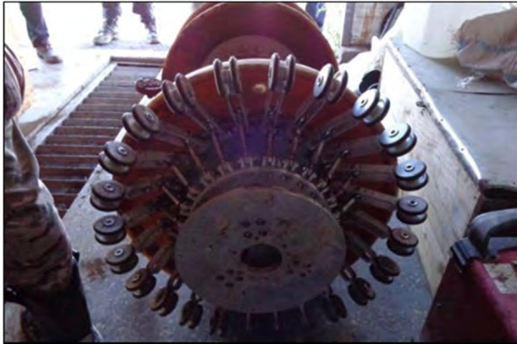
Intelligent caliper pig, Gori-Kareli pipeline segment
