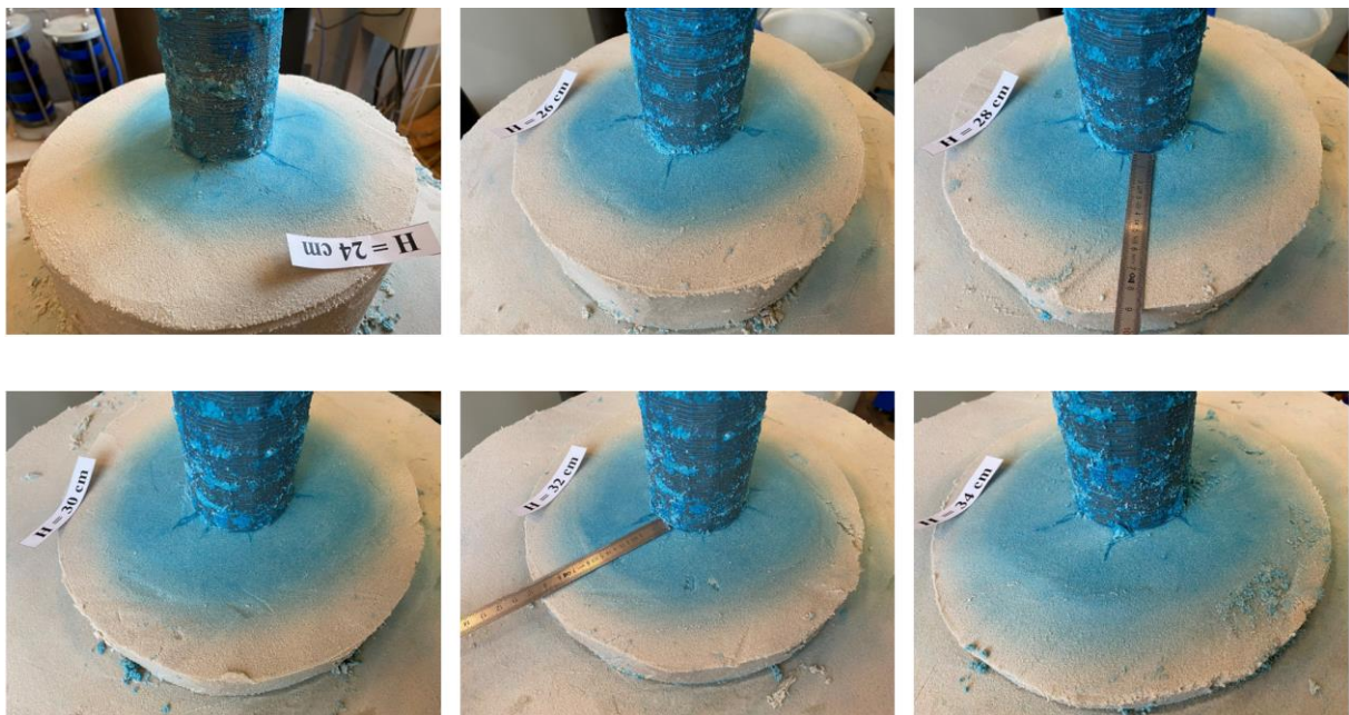
Figure 3.36: Test N33 - Transversal cross-sections of the inner ring at different heights (photos taken by a smartphone)
