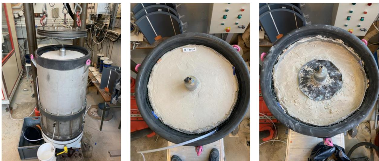
Fig. E-31: Excavation of the low permeability layer (sand pack N32).
