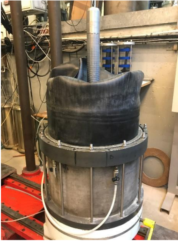
a – fixing the membrane onto the lower baseplate
