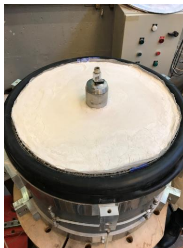
h – compaction of the upper low permeability layer
