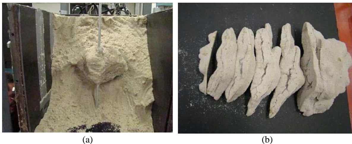
Figure 1.42: (a) invaded zone after solidifying of a typical specimen; (b) verticals cross-sections of the invaded zone chamber (Golovin et al., 2011).
