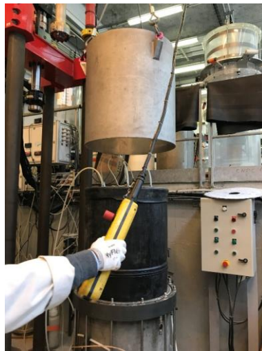
l – setting up the lateral confining cell
