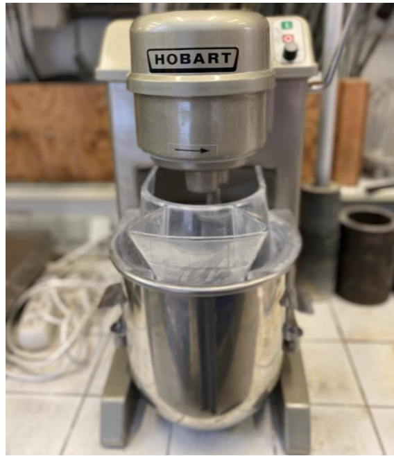
Figure 2.4: Mixer used for preparing the sand and fines mixture.
