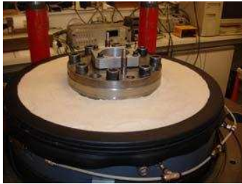
Figure 2: View of an open cell with the sand sample surrounding the metallic cylinder.
