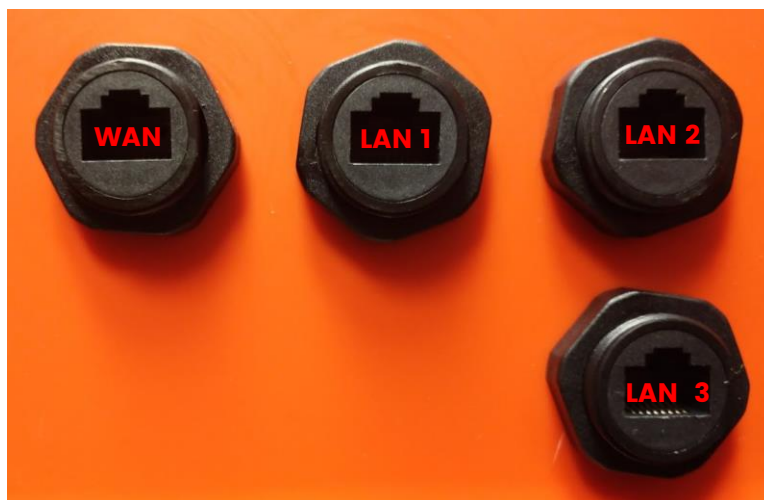
Figure 11: Connect the router to the RJ-45 ports on the case using ethernet cords.
