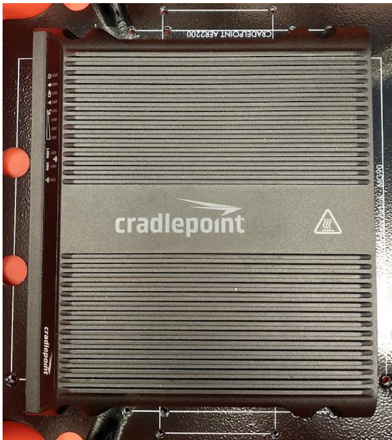
Figure 5: Mount the router to the base plate using PTA0399-TL screws.
