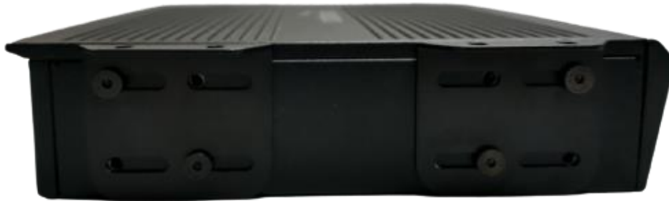
Figure 4: For AER2200 and E3000 routers, fasten the router mount brackets to the sides of the router using eight M4 screws.
