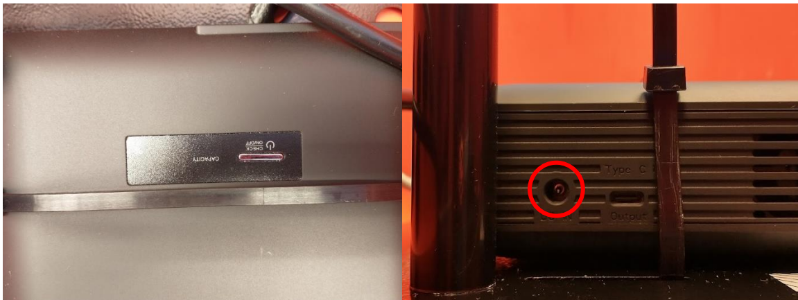
Figure 3: Ensure that the battery display and charging port are not covered by the cable tie.
