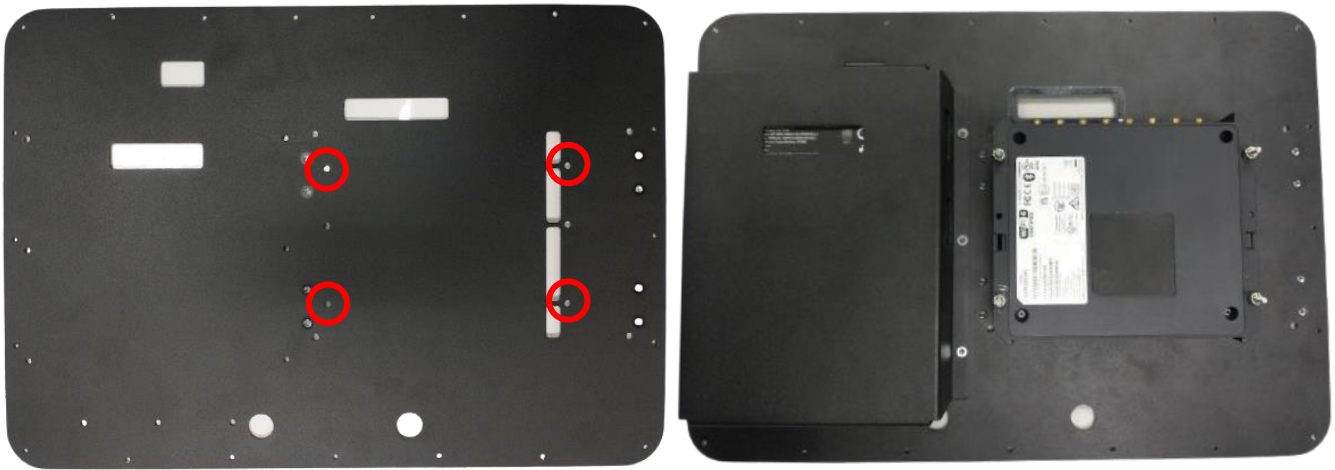
Figure 9: For R1900 router, fasten the router to the cover plate using PTA0579 screws and PTA0604 nuts.
