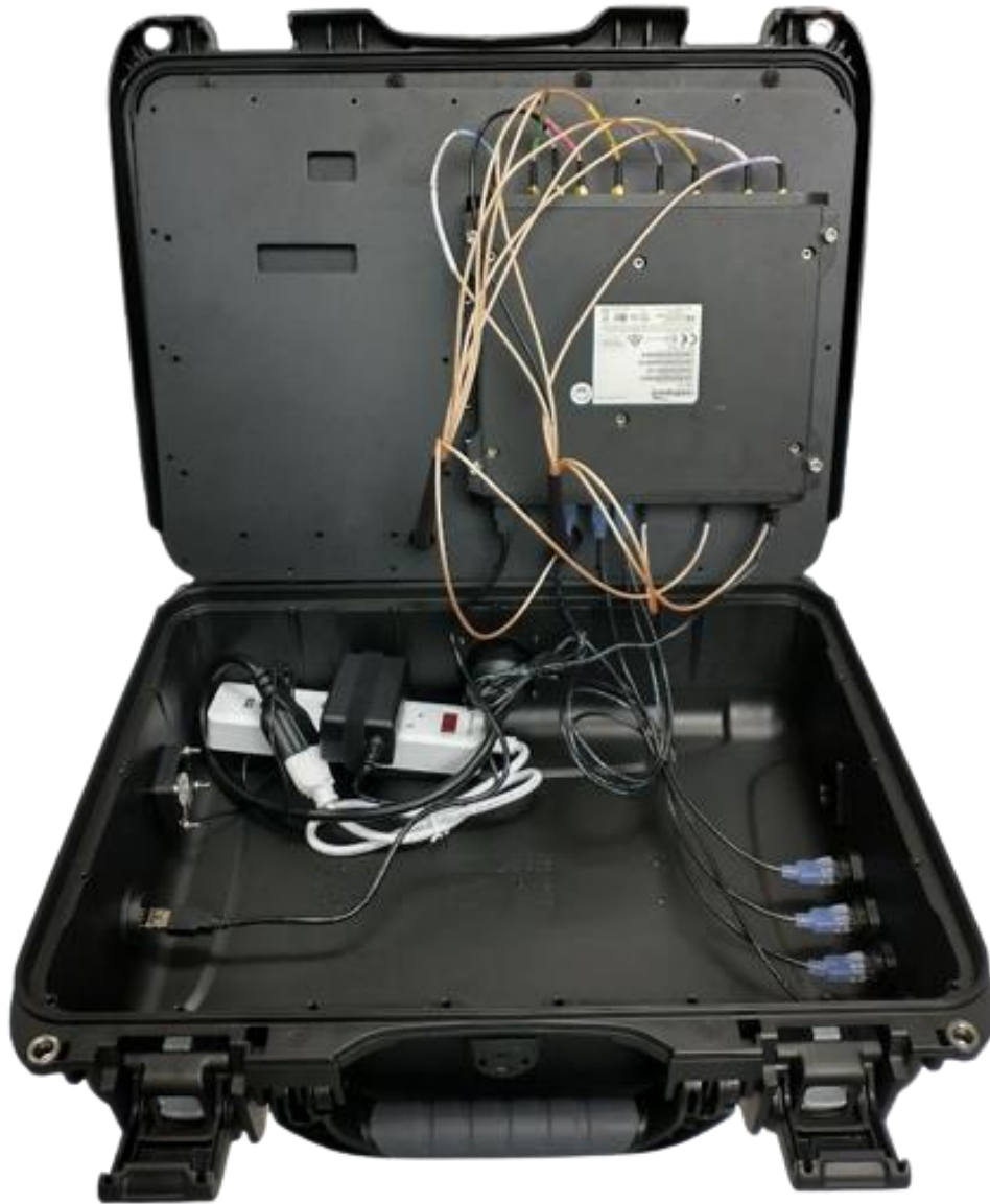
Figure 19: Fully Connected 13in1 Bloodhound L with Cradlepoint IBR1700 Router
