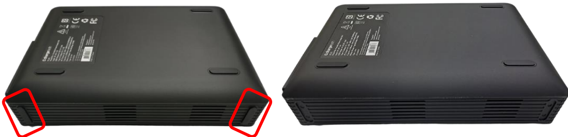
Figure 1: For the 54K battery, remove the pads from the bottom and side of the battery pack.
