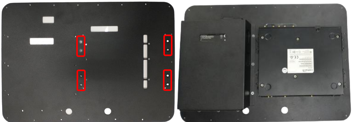
Figure 7: For AER2200 router, fasten the router to the cover plate using PTA0399-TL screws.
