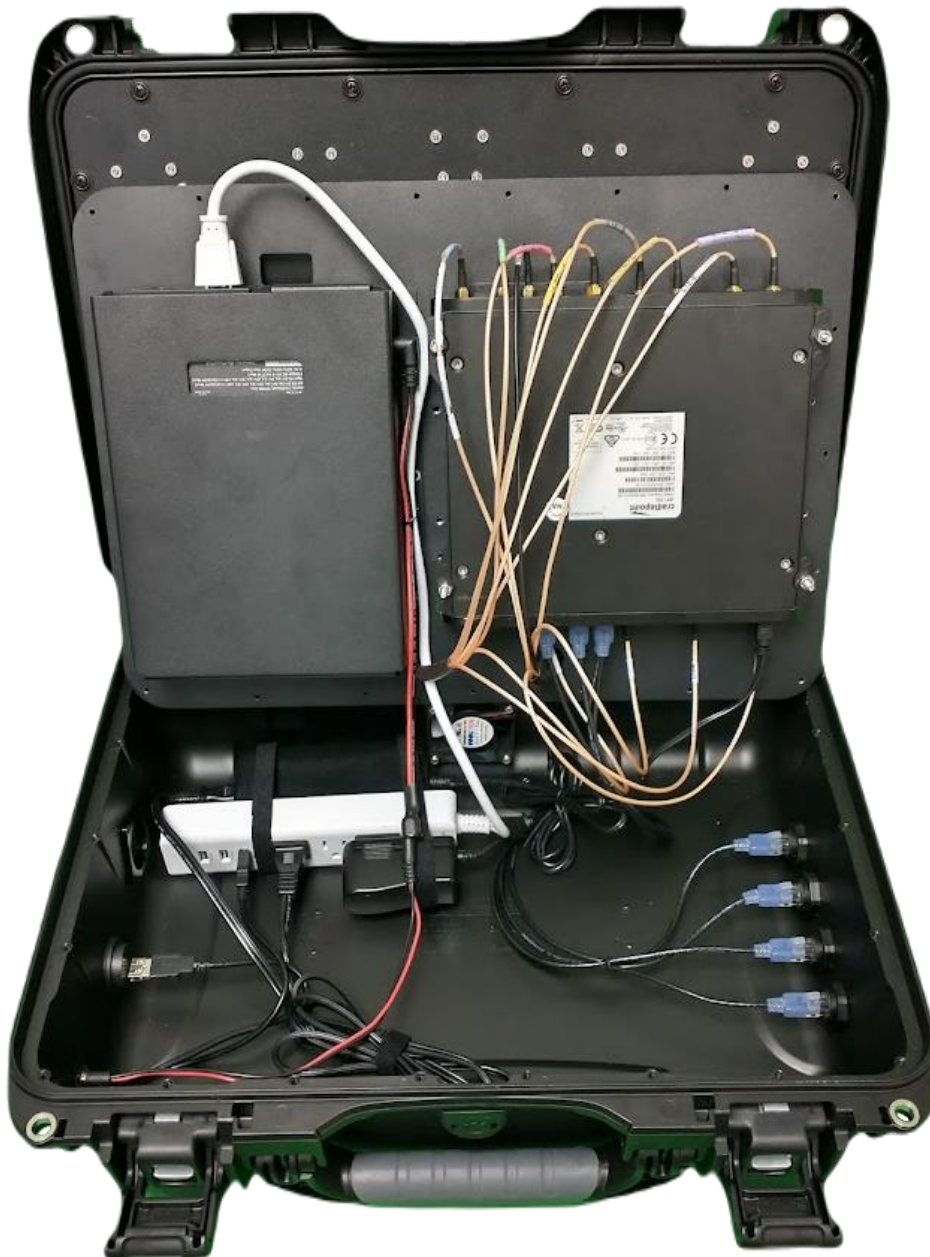
Figure 18: Fully Connected 13in1 Bloodhound G with Cradlepoint IBR1700 Router
