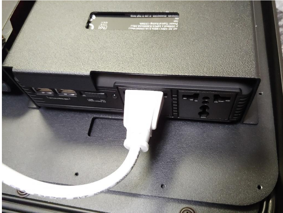
Figure 12: Insert the AC plug of the surge protector to the AC port of the battery.
