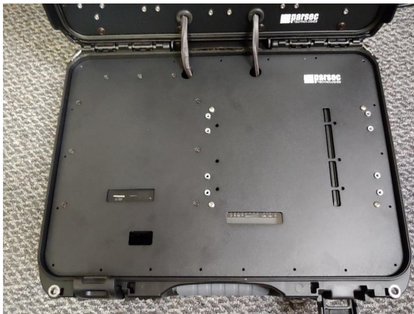
Figure 16: Fasten top cover plate to enclosure using black screws provided.
