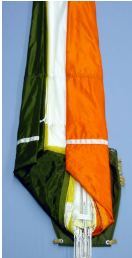
Figure 11 Folding the canopy : stage 4
