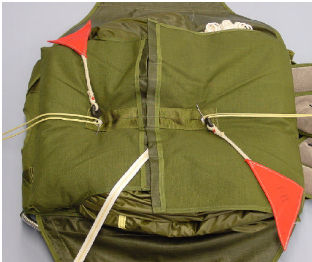
Figure 22 Closing the container : stage 1
