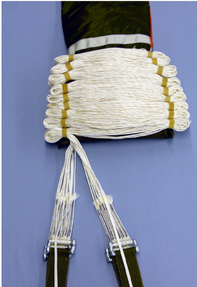
Figure 15 Diaper closed rigging lines stowed
