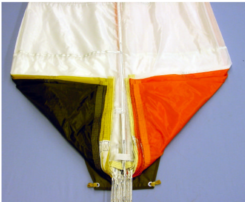
Figure 9 Folding the canopy : stage 2
