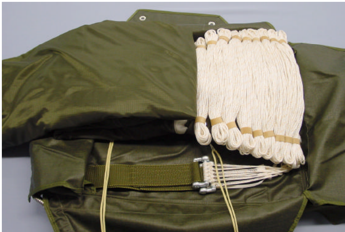
Figure 19 Stowing the canopy : first fold
