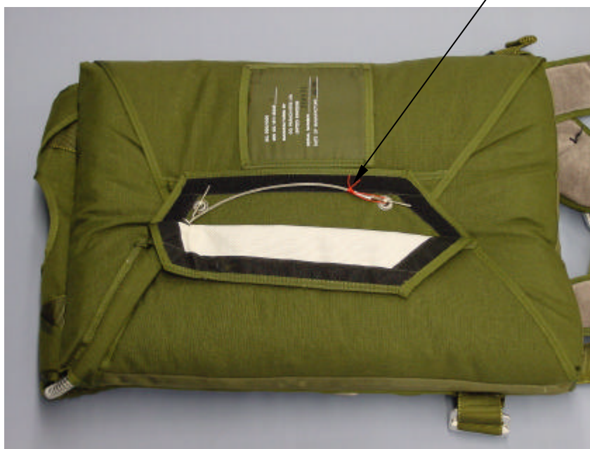
Figure 27 Container closed ripcord pins fitted
