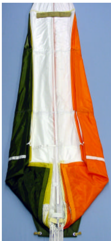
Figure 10 Folding the canopy : stage 3
