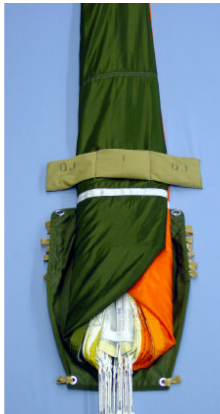
Figure 11 Folding the canopy : stage 4
