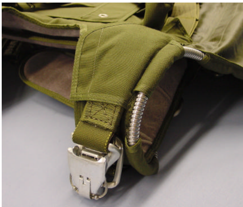
Figure 17 Riser covers secured
