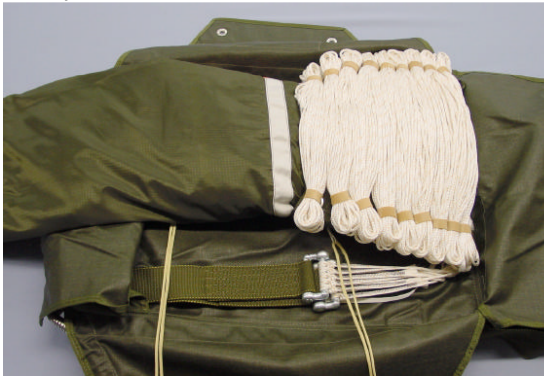
Figure 18 Risers and diaper positioned
