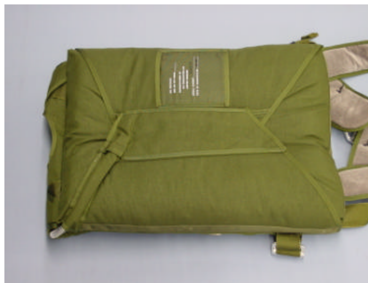
Figure 27 Container closed ripcord pins fitted
