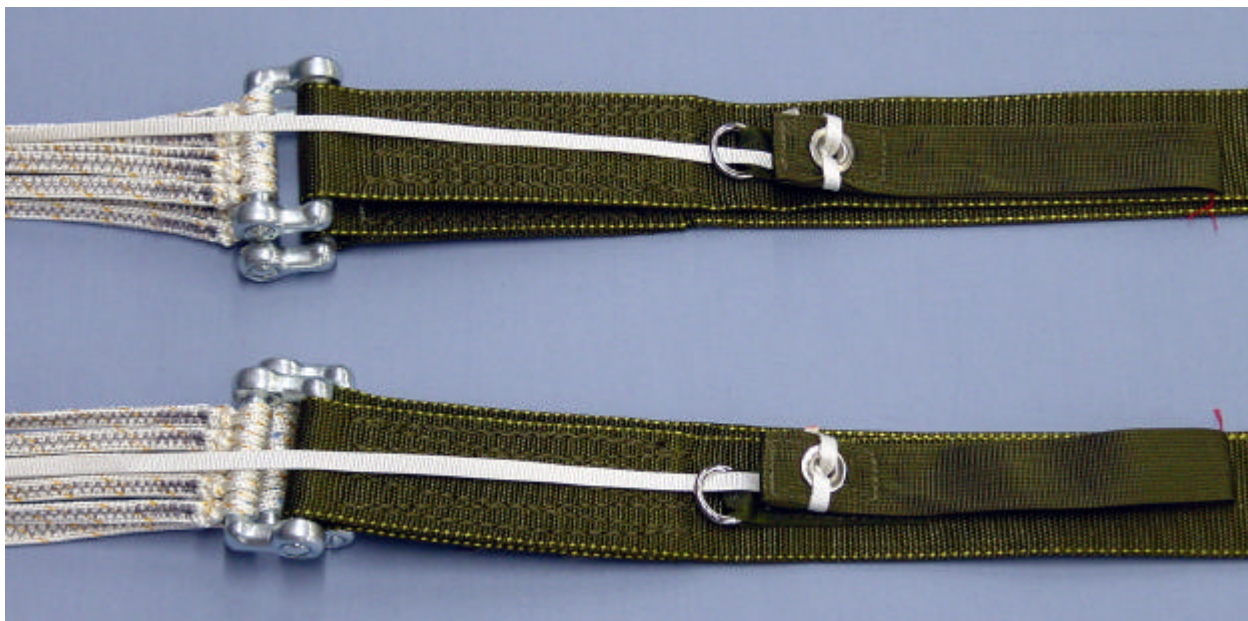
Figure 7 Securing the steering line handles to risers
