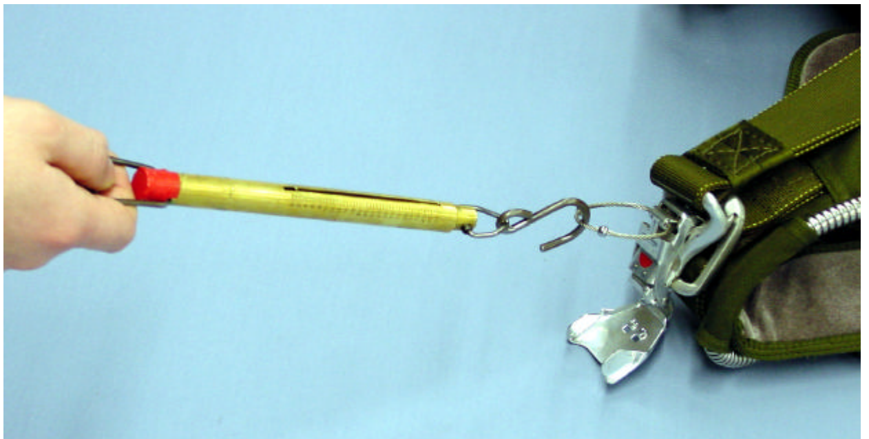
Fig 2 Capewell release : wire initiating latch test
