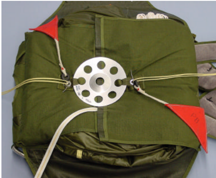
Figure 23 Positioning the kicker plate
