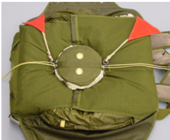
Figure 24 Pilot chute compressed
