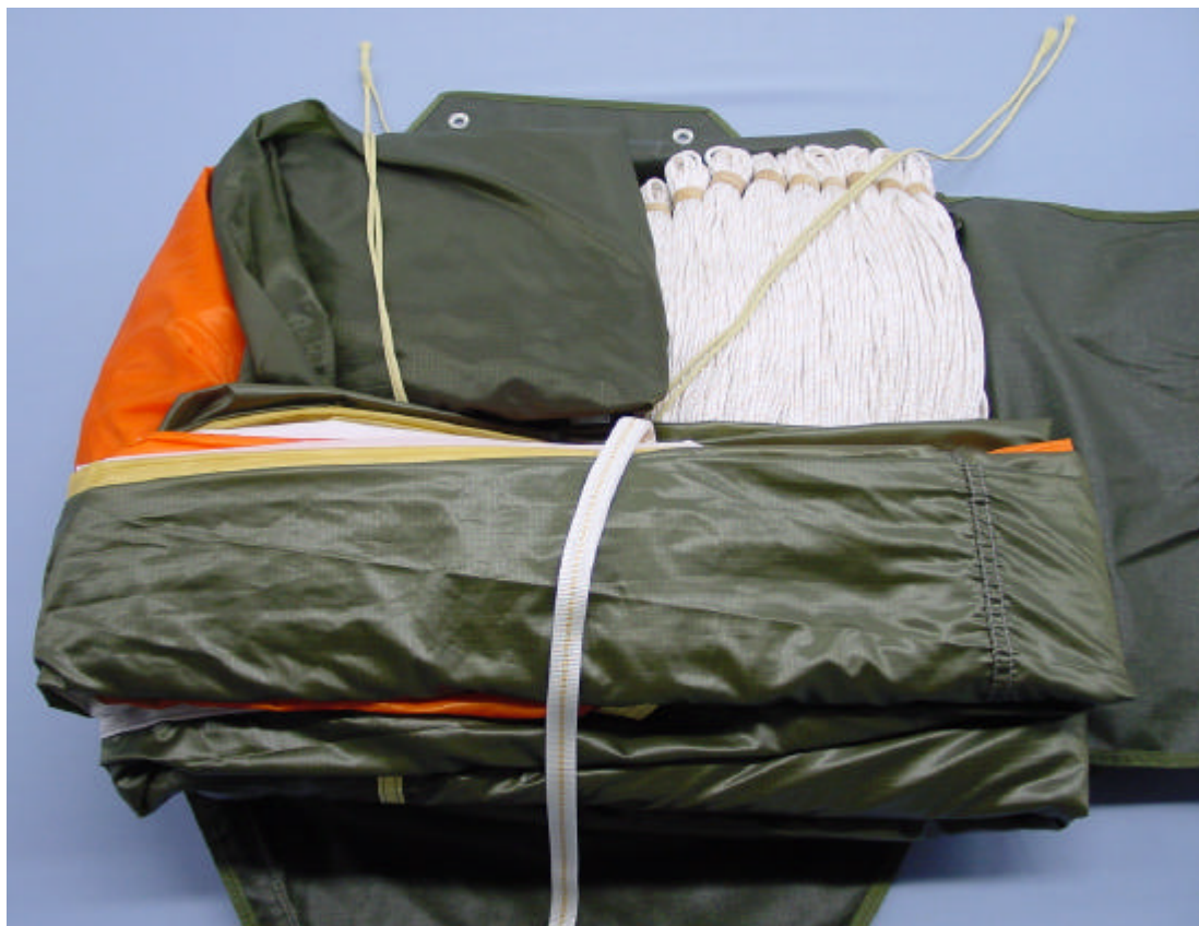
Figure 21 Stowing the canopy : final fold
