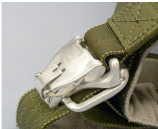
Figure 6 Connecting the Capewell shoulder releases
