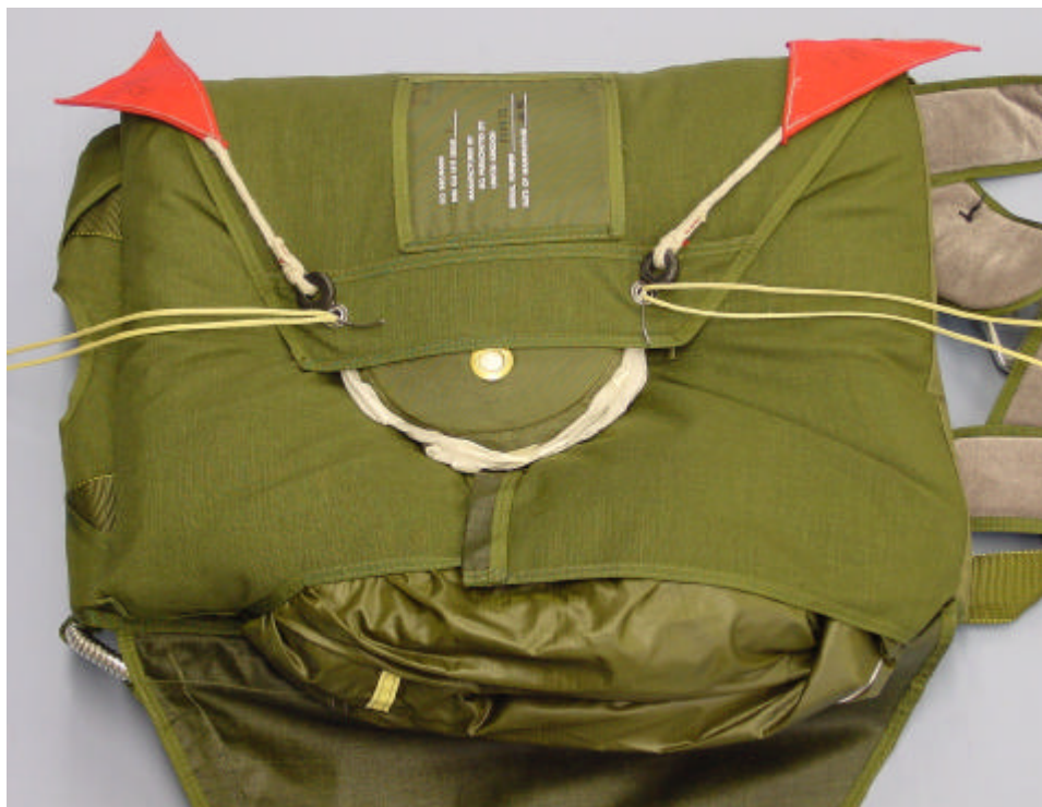
Figure 25 Closing the container : stage 2
