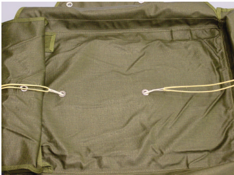
Figure 3 Fitting the closure loop
