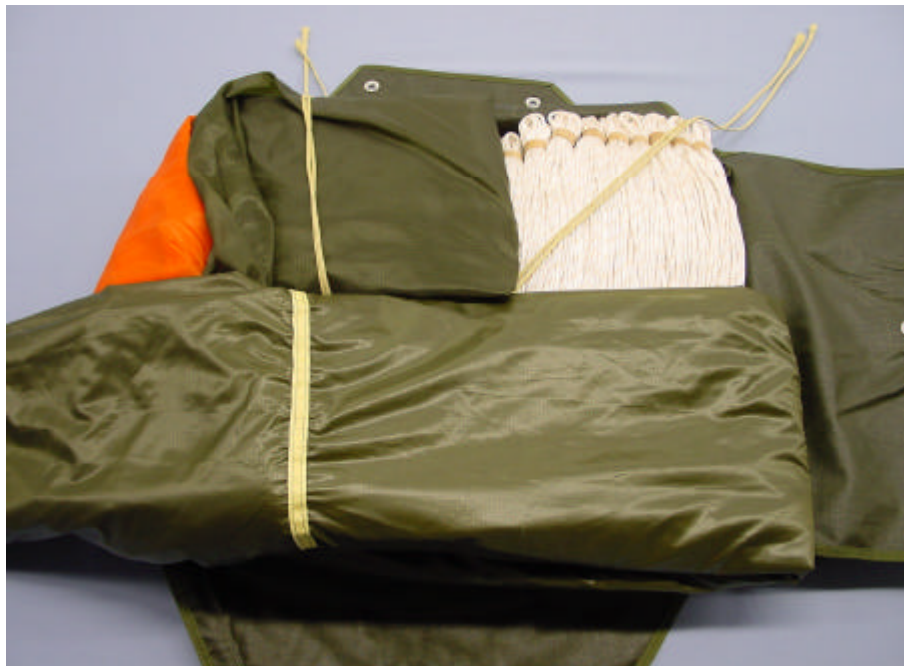
Figure 20 Stowing the canopy : second and third fold
