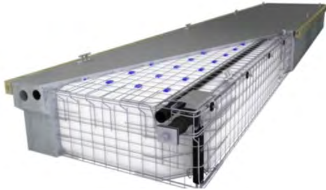
Concrete float concept design mockup
