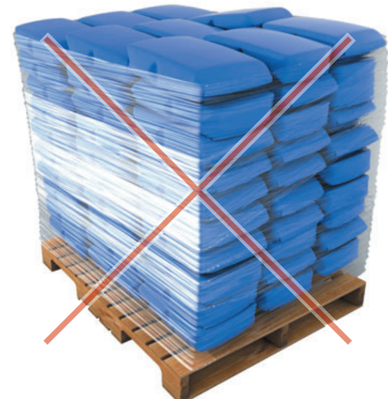
INCORRECT (Not interlocked, no bottom tray)
