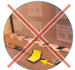
Pallet restraining devices that penetrate trailer flooring are NOT ALLOWED .
