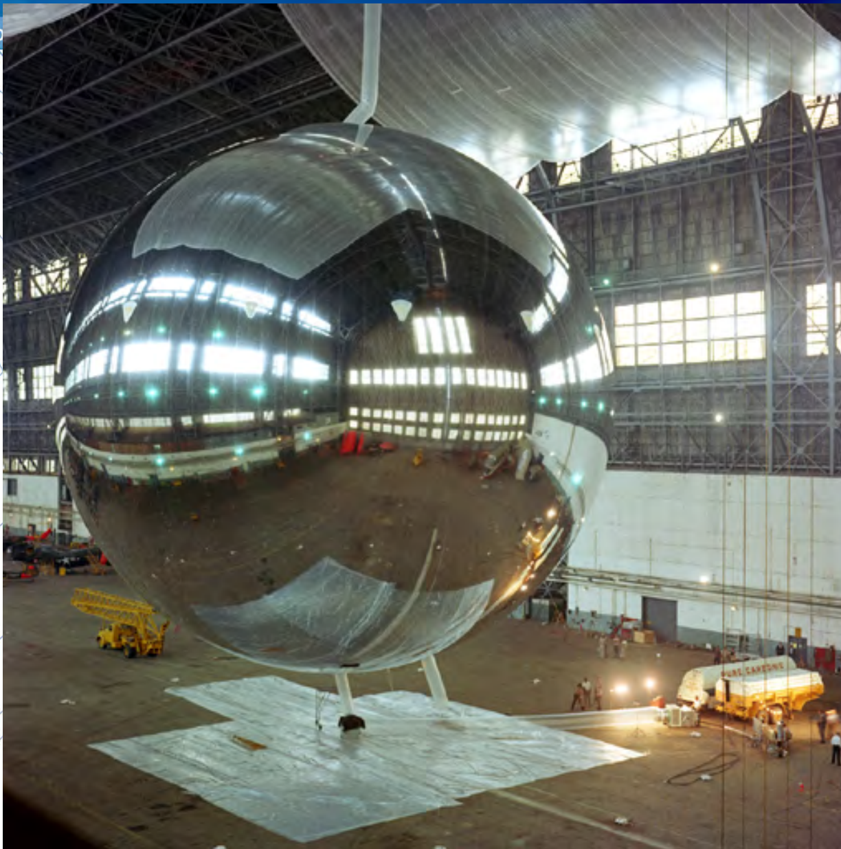
ECHO/PAGEOS Balloon Satellite National Oceanic and Atmospheric Administration type of satellite photographed by BC-4
