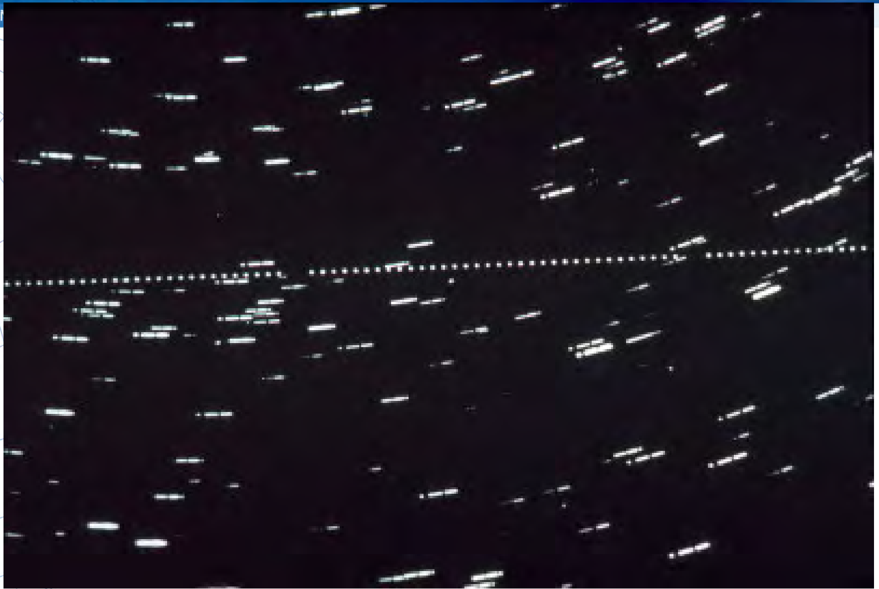
BC-4 camera photograph stars in circular pattern satellite is a series of dots in straight line.
