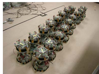
Fig. 7. Mobile robot integrated with silk moth brain
