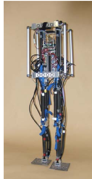
Figure 4: 3D biped robot with biarticular muscles
