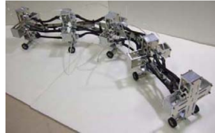
Fig. 5. Snake-like robot with pneumatic actuators
