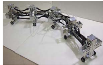
Figure 7 Snake-like robot with pneumatic actuators
