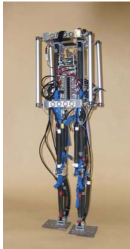
Fig. 3. Biped robot with biarticular muscles
