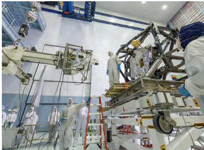
The ETIS II team is integrating the Mid-Infrared Instrument (MIRI) into the Integrated Science Instrument Module (ISIM) at Goddard Space Flight Center.
