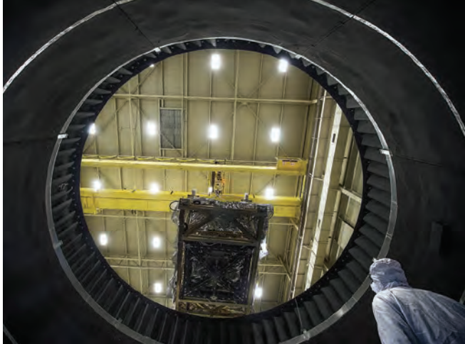
A component of JWST lowers into NASA GSFC's Space Environment Simulator.
