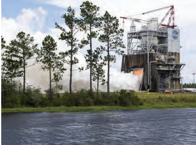
Test of a RS-25 Engine Controller on the A-1 Test Stand at Stennis Space Center.
