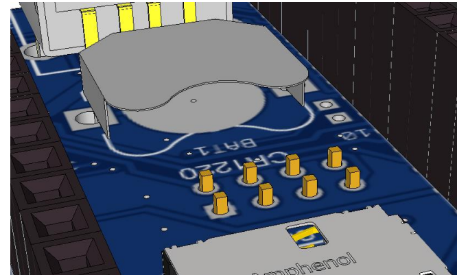
Figure 2 Wi-Fi Header Incorrect Installation
