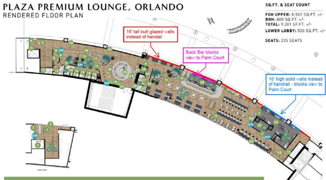
Figure 4: Trip Plan showing glazed wall and back bar blocking views of Palm Court
