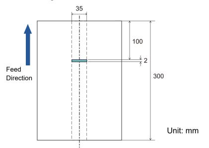
Since the detection range (length) is less than 5 mm, multifeeds cannot be detected accurately.
