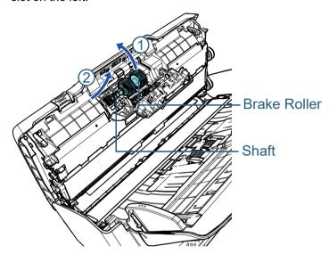
4 Remove the brake roller from its shaft.
