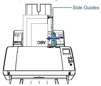
8 Scan the documents with the image scanning application. For details, refer to the image scanning application manual.
