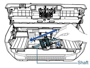
2 Rotate the bushing on the shaft in the direction of the arrow.
