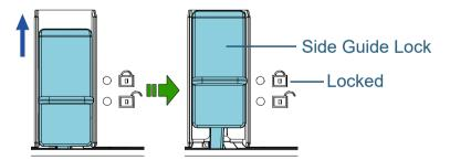
7 Adjust the other side guide to the target position.
