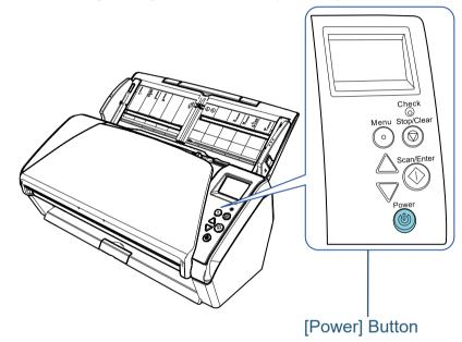
⇒ The scanner is turned on, and the [Power] button lights in green. During initialization, the following image is displayed on the LCD of the operator panel.
