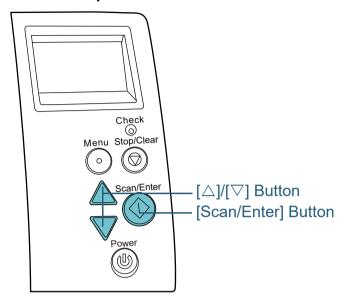
**1** Press the  $[\triangle]$  or  $[\nabla]$  button while the [Ready] screen is displayed on the operator panel.
