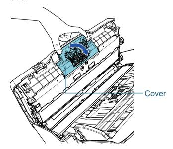
2 Lift the right side of the roller first, then pull out the shaft from the slot on the left.
