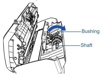
3 Close the sheet guide. Make sure that both ends of the sheet guide are locked firmly.
