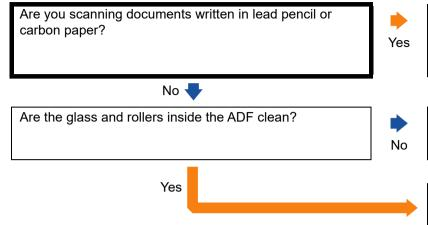
When you scan documents written in lead pencil, make sure to clean the rollers frequently. Otherwise, the rollers will be contaminated which may leave black traces on the document or cause feeding errors.
