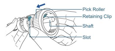
2 Insert the retaining clip of the other pick roller into the slot.
