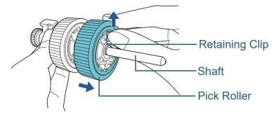
2 Pull out the other pick roller from the shaft as you lift the retaining clip.
