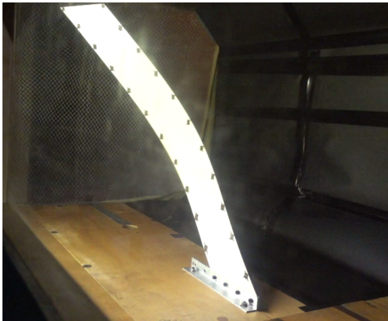
(b) Snapshot of the plate motion in the wind tunnel ( U = 13.8 \text{ m/s} = 1.03U_f^{\text{exp}} ).
