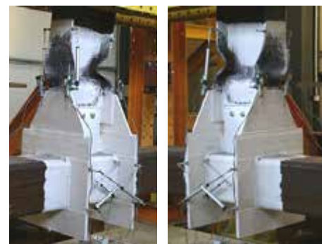
Figure 4.109. S460-CP-C joint: cyclic response & illustration of failure mode
