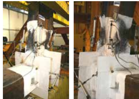
Figure 4.104. S460-RBS-M joint: monotonic response & illustration of failure mode
