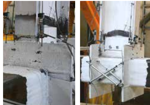
Figure 4.112. S460-RBS-R-M joint: monotonic response & illustration of failure mode
