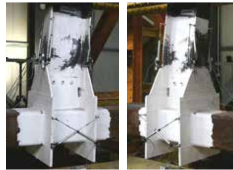
Figure 4.108. S460-CP-M joint: monotonic response & illustration of failure mode
