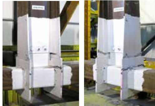
Figure 4.119. S700-CP-R-C joint: cyclic response & illustration of failure mode
