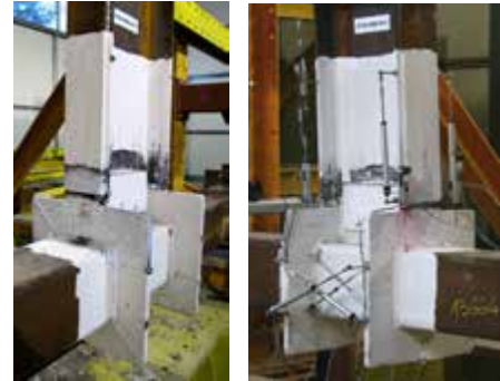
Figure 4.115. S700-RBS-R-C joint: cyclic response & illustration of failure mode
