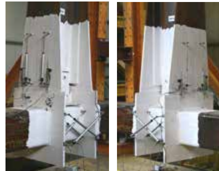
Figure 4.116. S460-CP-R-M joint: monotonic response & illustration of failure mode
