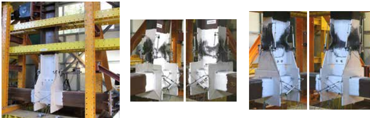
Figure IX. Experimental investigation of welded beam-to-column joints (Univ. of Timisoara)
