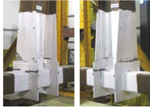
Figure 4.118. S700-CP-R-M joint: monotonic response & illustration of failure mode
