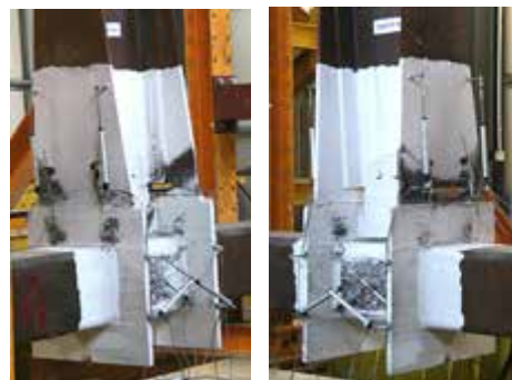
Figure 4.117. S460-CP-R-C joint: cyclic response & illustration of failure mode
