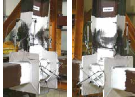
Figure 4.107. S700-RBS-C joint: cyclic response & illustration of failure mode
