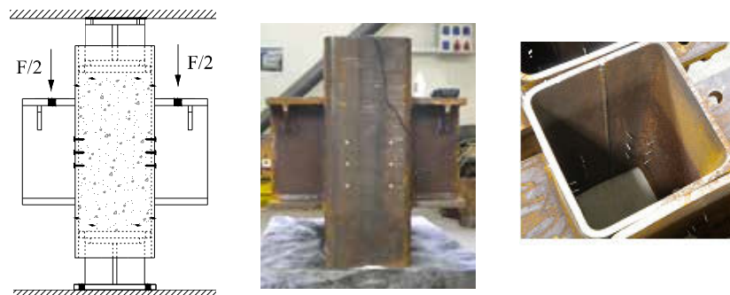
Figure 4.96. Specimen configuration for the load introduction tests
