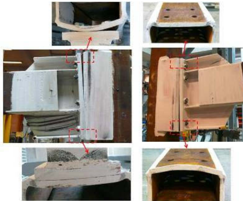
Figure 4.67. Failure mode of the B-EP-U joints (reverse U channels yielded)
