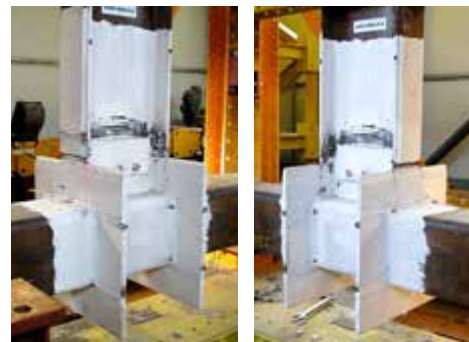
Figure 4.113. S460-RBS-R-C joint: cyclic response & illustration of failure mode
