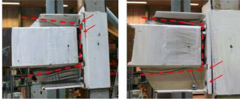
Figure 4.66. B-EP-H joint – failure in the connection (4 bolts in the tension zone failed and the hammer head in compression yielded)
