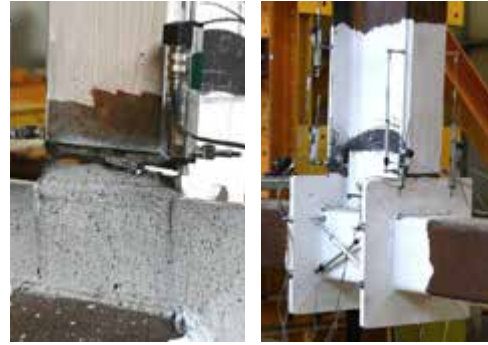
Figure 4.114. S700-RBS-R-M joint: monotonic response & illustration of failure mode
