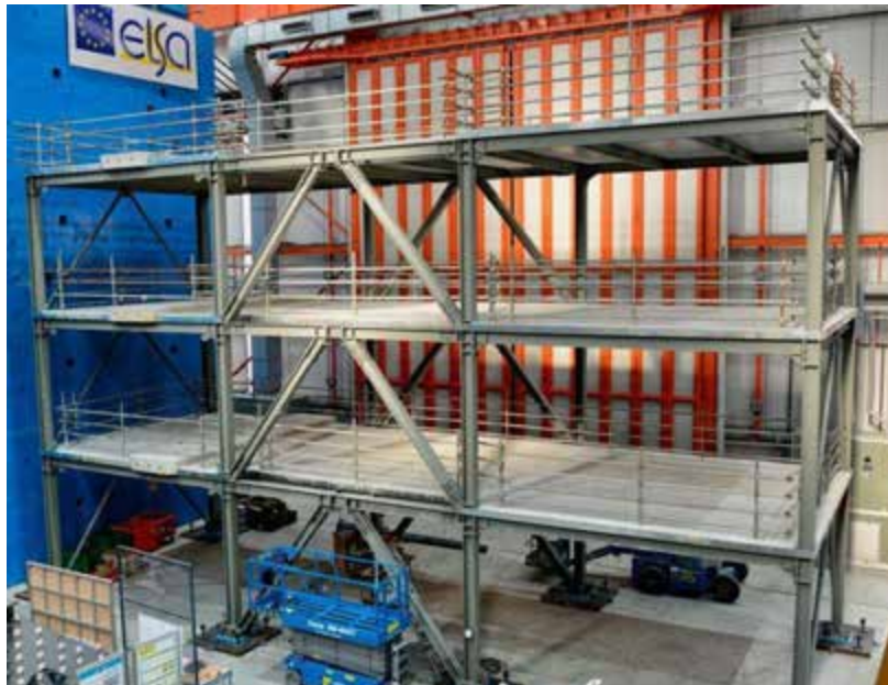
Figure XV. Full-scale experimental validation of dual eccentrically braced frame with removable links
