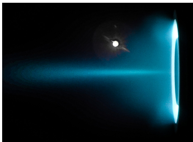
FIG. 22. Photograph of PSAC/SPCS miniaturized Hall thruster firing at 0.5 \text{ mg s}^{-1} of Xe supply. The typical characteristics of the cathode with krypton discharge are listed in Table VII.
