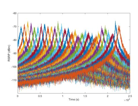
Fig. 2. Received signal strength in a legitimate scenario.
