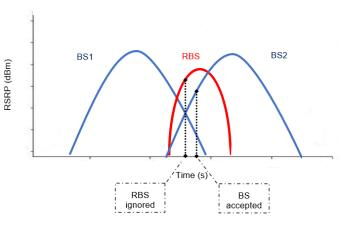
Fig. 5. Detection of rogue base stations and transfer to a legal base station.
