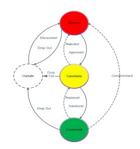
Fig. 8. BS state machine in Analyser.
