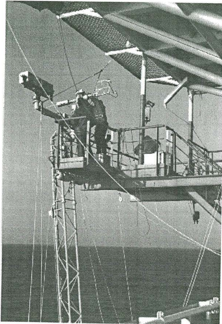
Figure 6-2 Instrument boom with RSSG and other instruments
