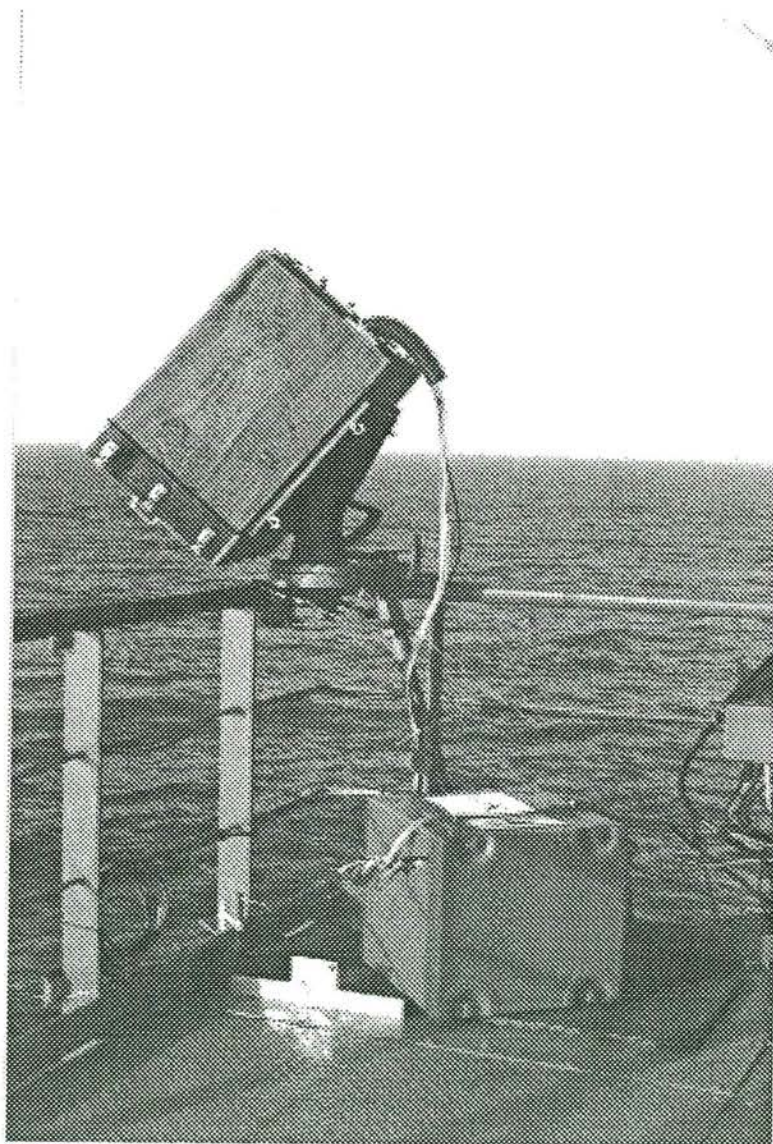
Figure 6-21 The FM-CW X-band scatterometer at MPN
