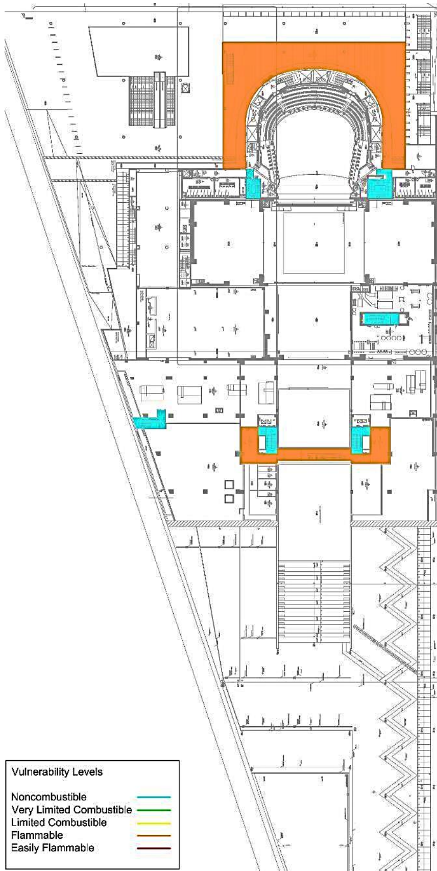
Figure D-11 Third floor finishing material vulnerability (Scale ~ 1/1000)
