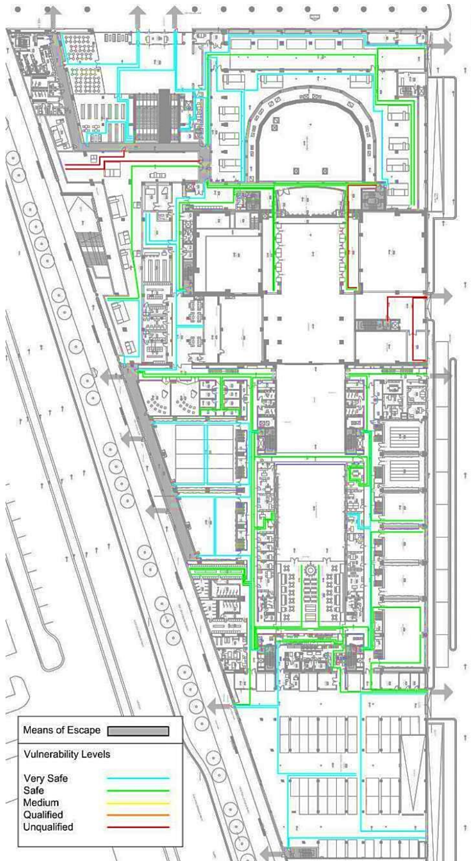
Figure 4.5 Ground floor means of escape vulnerability (Scale ~ 1/1000)
