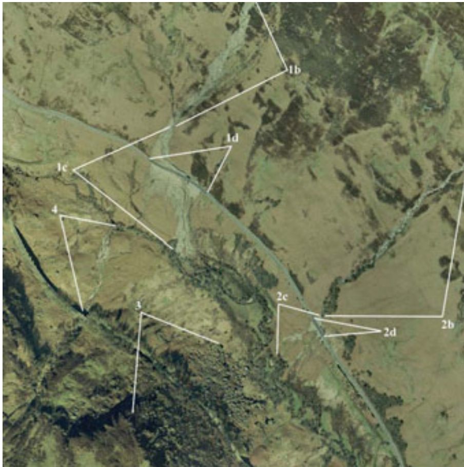
Figure 6.1 – Aerial photograph showing the northerly (N) and southerly (S) debris flows that occurred in Glen Ogle in August 2004 with key features marked. The photograph represents a 1km by 1km square; north is to the top.
