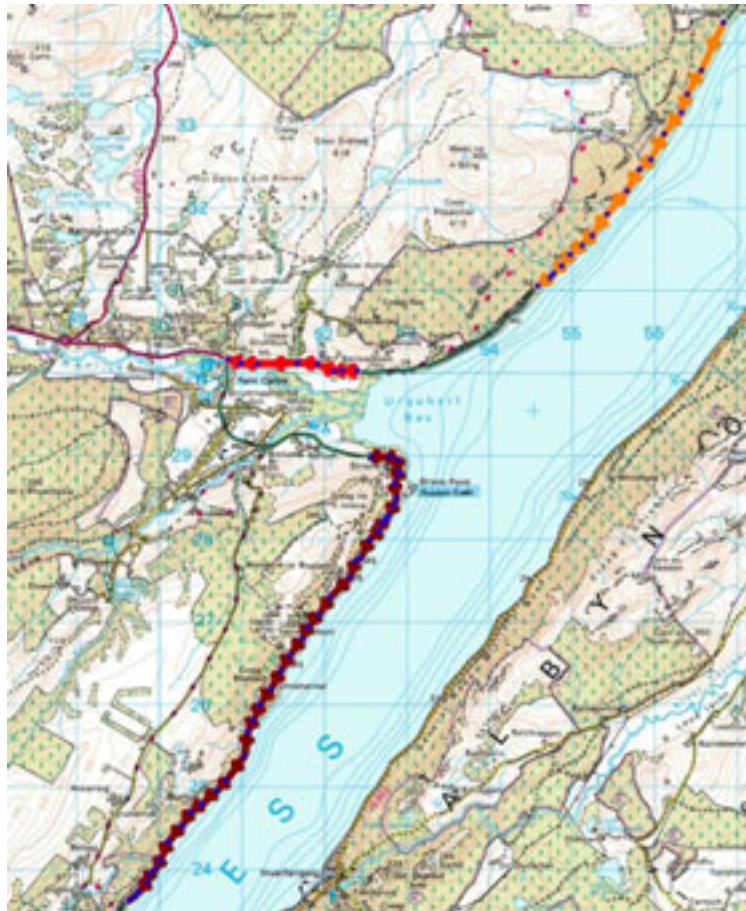
Figure 5.8 – Ordnance Survey two-dimensional imagery for A82 Loch Ness. Showing lengths categorised at Priority 3 (A82-03), Priority 1 (A82-04) and Priority 2 (A82-05) from top to bottom. Digital Ordnance Survey imagery at 1:50,000 is shown but the image itself is not to scale. (© Crown Copyright. All rights reserved Scottish Government 100020540, 2008.)
