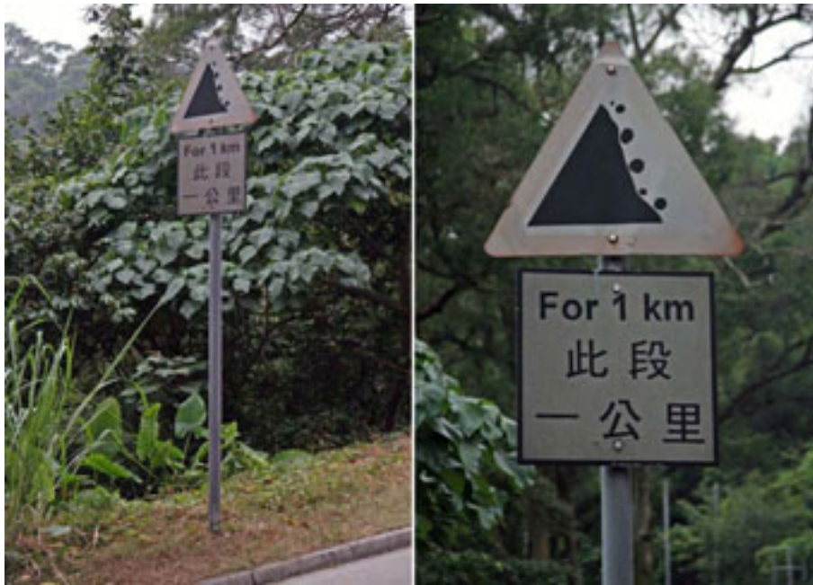
Figure E.10– Rockfall road sign in Hong Kong indicating the start of the hazard and the distance over which it is extant.
