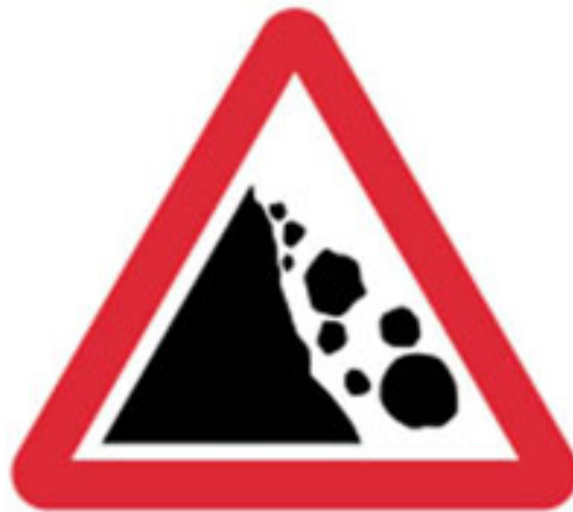
Figure 8.4 – UK rockfall sign (TSRGD, 2002: Diagram 559) indicating risk of falling or fallen rocks.
