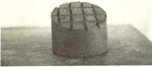
Figure 3. Bottom layer of a bond test specimen.
