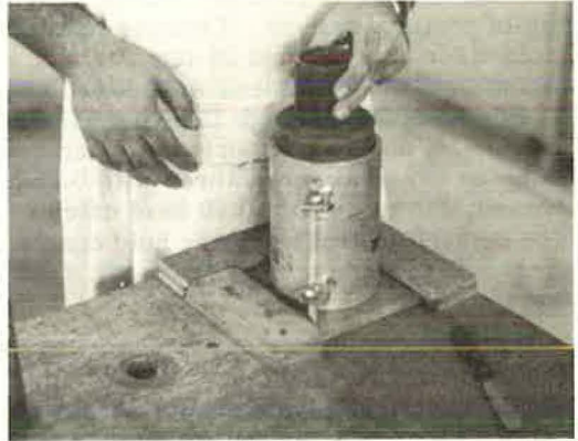
Figure 2. Finishing head fabricated to fit inside the compaction mold.
