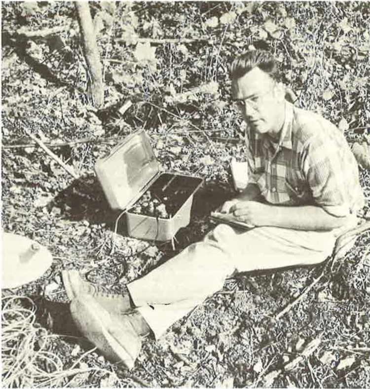
Figure 8. Geologist operating Model MD-1 engineering seismograph.
