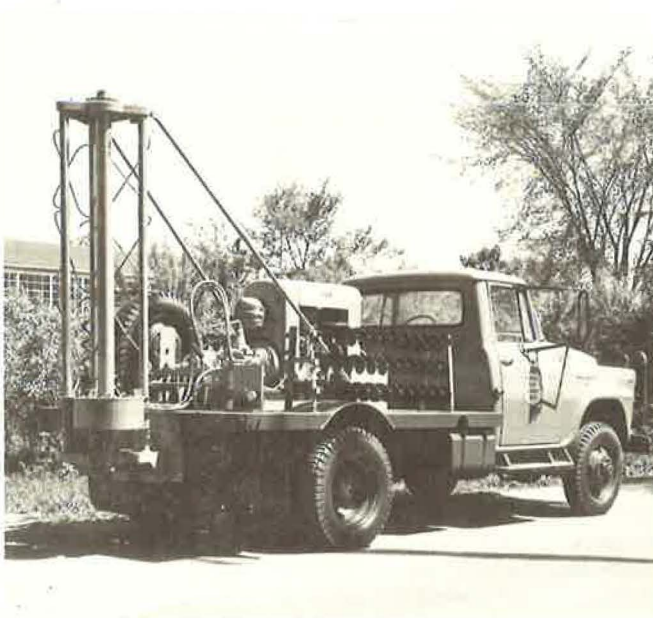
Figure 5. B-36 mobile drilling unit.
