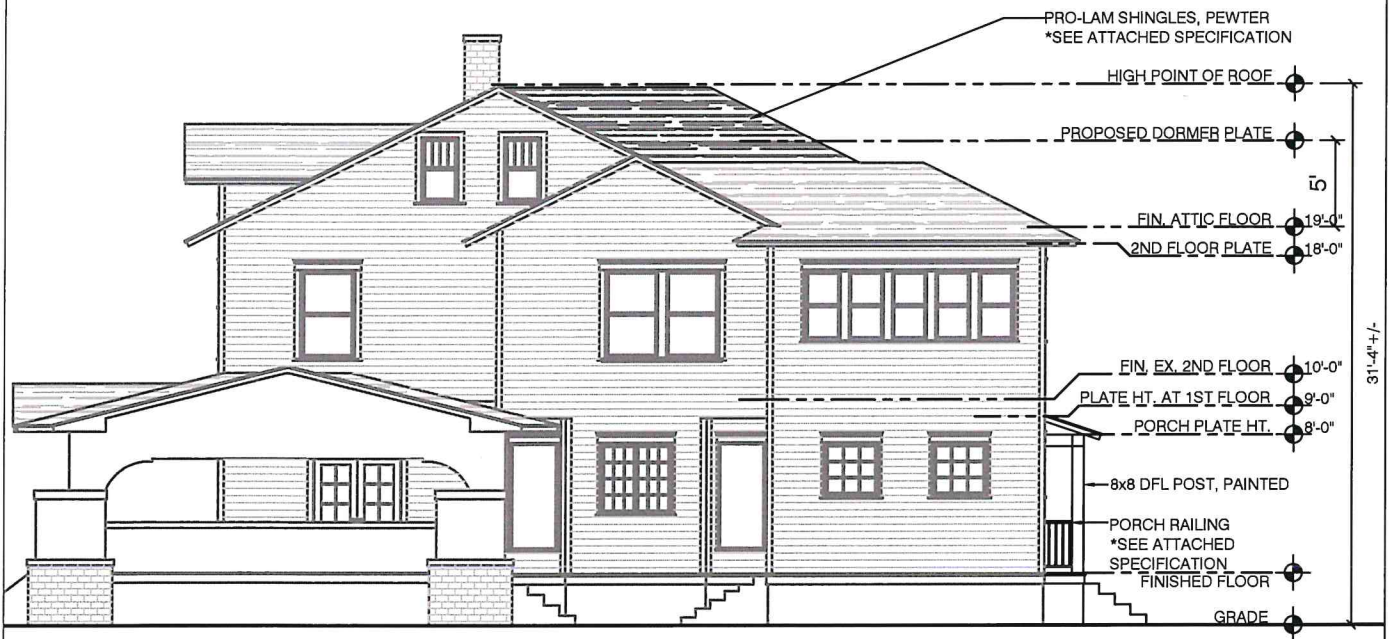
② EAST ELEVATION PROPOSED 3/32" = 1'-0"
