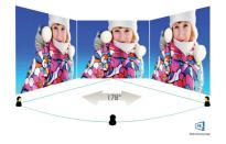
IPS displays use an advanced technology that gives you extra-wide viewing angles of 178/ 178 degrees, making it possible to view the display from almost any angle. Unlike standard TN panels, IPS displays give you remarkably crisp images with vivid colours, making them ideal not only for Photos, movies and web browsing, but also for professional applications that demand colour accuracy and consistent brightness at all times.
