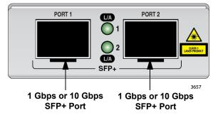
Figure 2. MMC10GSP/SP Front Panel
