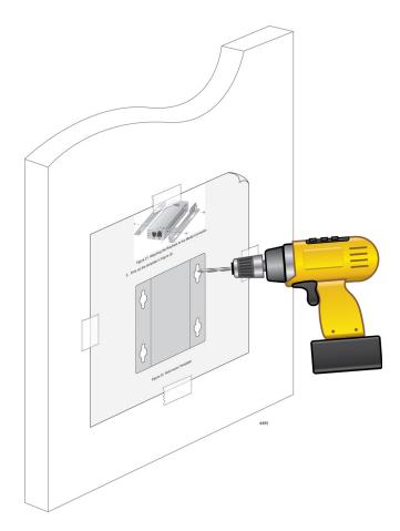
Figure 33. Placing the Template on the Wall
