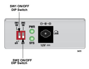
Figure 9. Media Converter Back Panel
