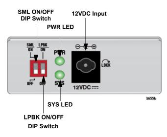
Figure 4. Alternate Media Converter Back Panel
