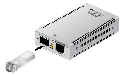
Figure 35. Inserting the SFP
