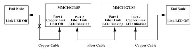
Figure 16. SML with Copper Connection Down in Two Media Converters Configuration
