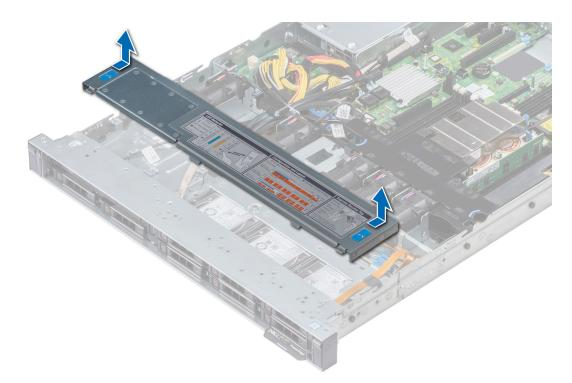
Figure 22. Removing backplane cover
