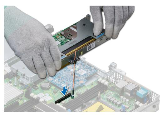
Figure 56. Installing an expansion card riser 1
