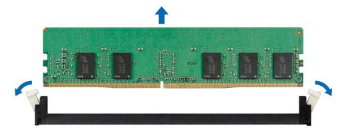
Figure 41. Removing a memory module
