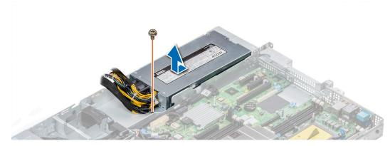
Figure 101. Removing non-redundant cabled AC PSU
