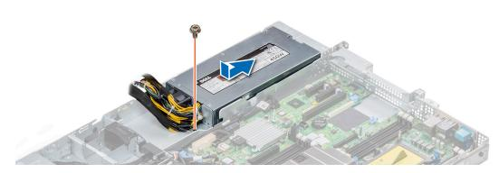
Figure 102. Installing a non-redundant cabled AC PSU
