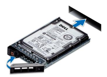
Figure 37. Installing a hard drive
