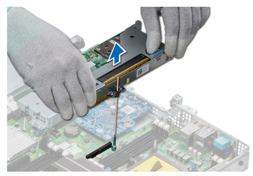
Figure 59. Removing an expansion card riser 1
