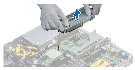
Figure 60. Removing an expansion card riser 2
