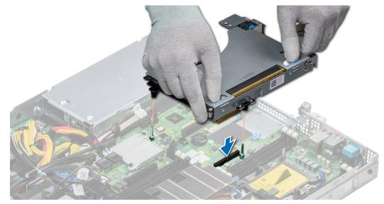
Figure 55. Installing an expansion card riser 1A
