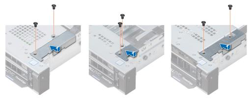
Figure 110. Installing the cable cover
