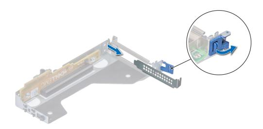
Figure 65. Removing filler bracket for riser 2
