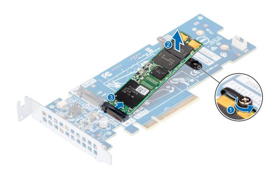
Figure 76. Removing the M.2 SSD module
