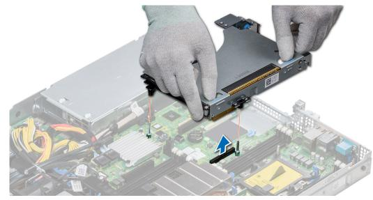
Figure 58. Removing an expansion card riser 1A
