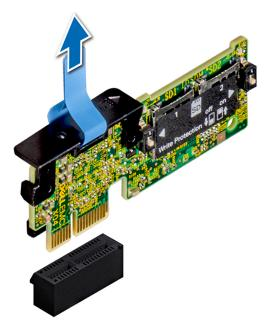
Figure 79. Removing the optional IDSDM/vFlash card
