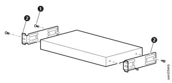
Secure the appliance to the rack, using cage nuts and screws (not provided).
