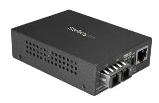
This fiber media converter converts and extends a Gigabit Ethernet fiber (1000 Mbps) network up to 10 km over single-mode fiber on 1000BASE-LX networks.
