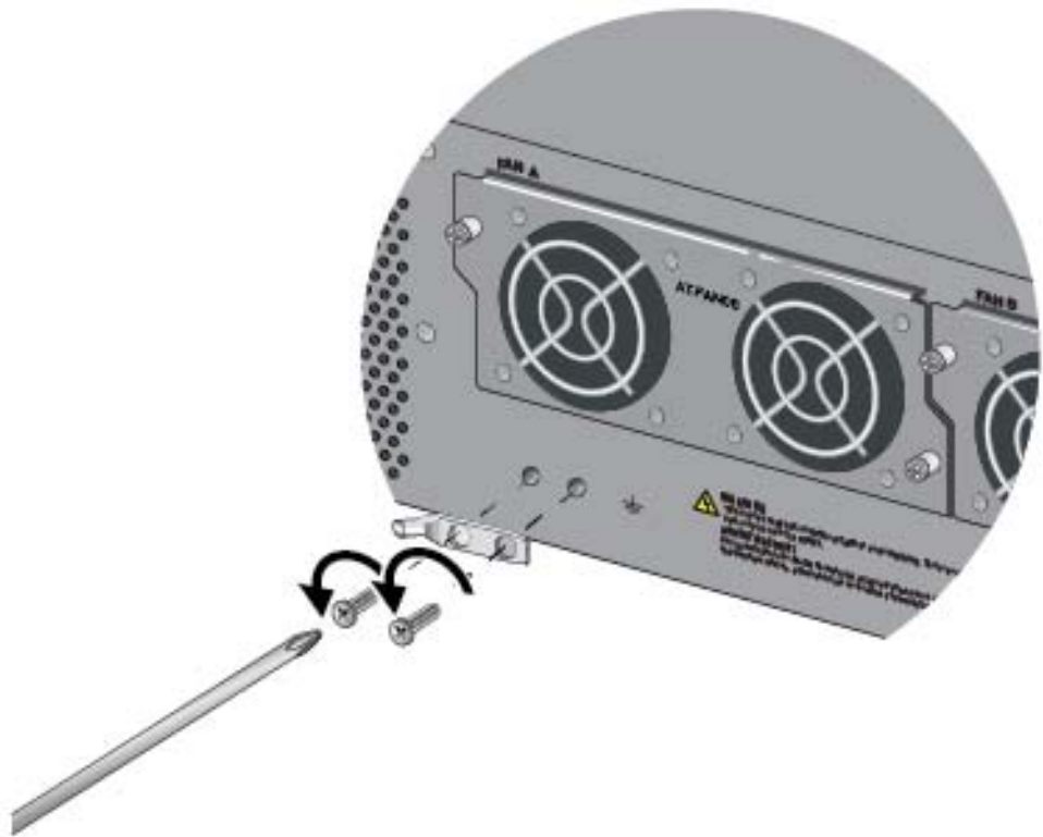
Figure 24. Removing the Grounding Lug from the Chassis
