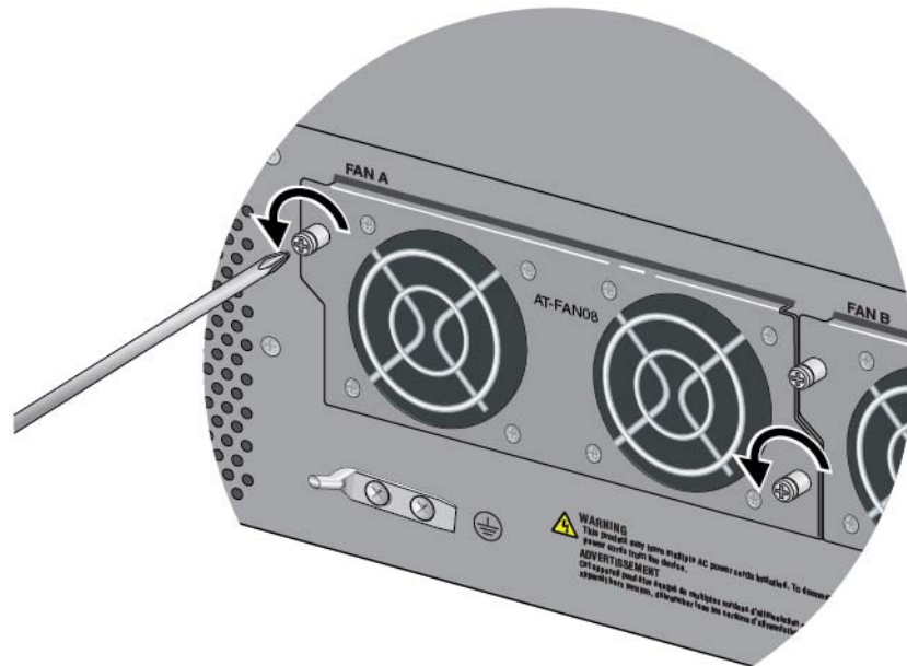
Figure 111. Loosening the Screws on the AT-FAN08 Module
