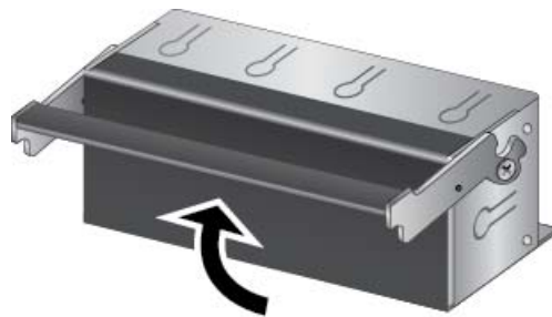
Figure 43. Lifting the Locking Handle on the Blank Power Supply Slot Cover
