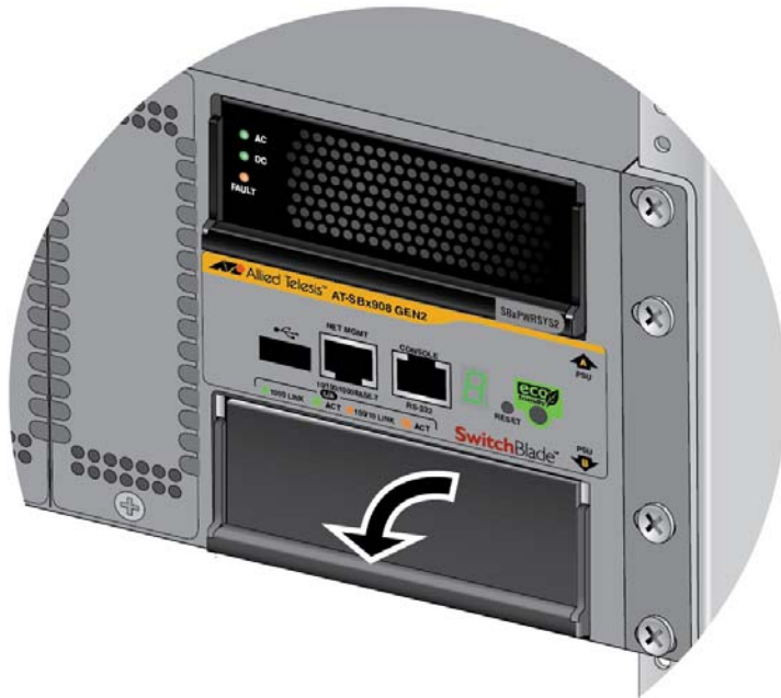
Figure 45. Lowering the Locking Handle on the Blank Power Supply Slot Cover
