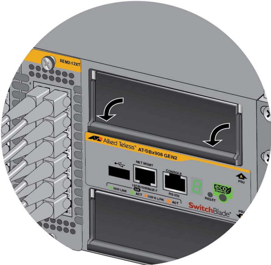
Figure 106. Lowering the Locking Handle on the Power Supply Slot Cover
