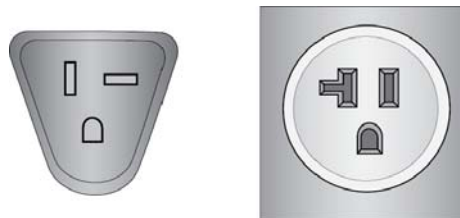
Figure 9. NEMA 5-20P Plug and Receptacle
