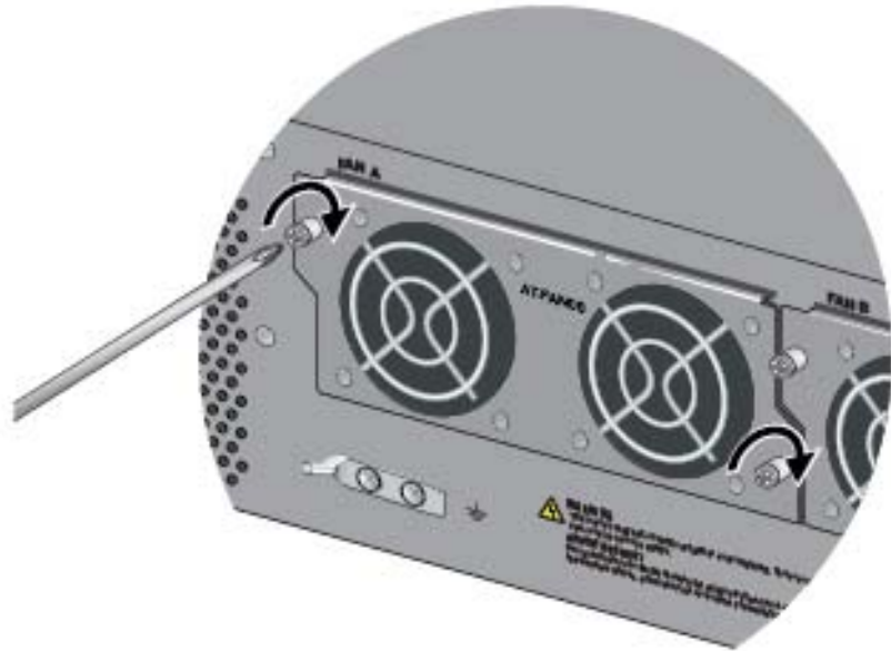
Figure 115. Tightening the Two Captive Screws on the AT-FAN08 Module
