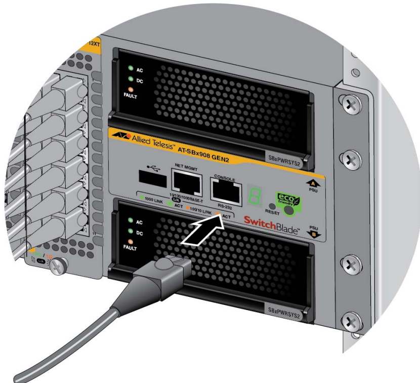
Figure 83. Connecting the Management Cable to the Console RS-232 Port
