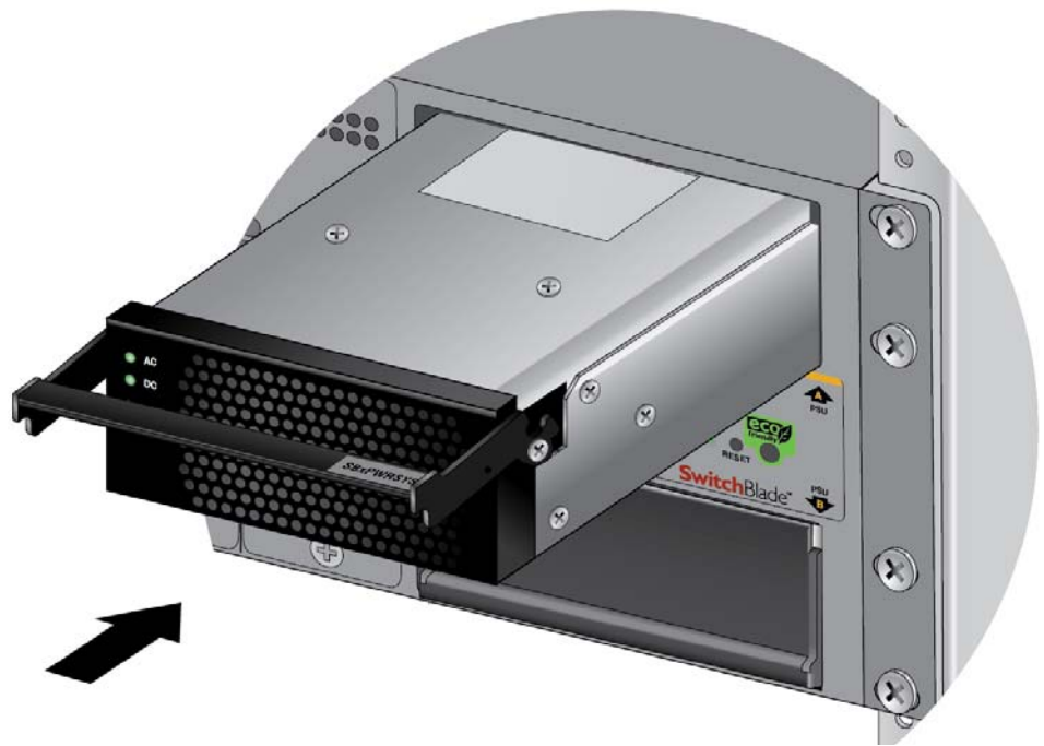
Figure 29. Sliding the AT-SBxPWRSYS2 AC Power Supply into the Chassis
