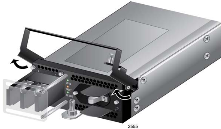
Figure 33. Lifting the Locking Handle on the AT-SBxPWRSYS1-80 DC Power Supply
