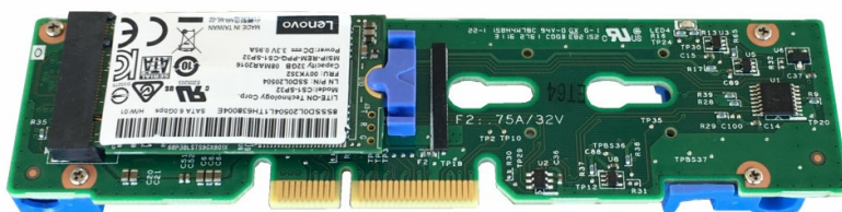
Figure 5. Single M.2 Boot Adapter and a 32 GB M.2 drive
