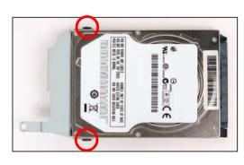
3. Lay the HDD or SSD into its drive bay and push it gently to the right
