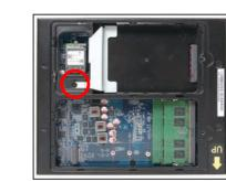
Place the HDD or SSD in the rack and secure with two screws from each side
