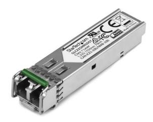
The GLCZXSMRGDST is a Cisco GLC-ZX-SM-RGD compatible fiber transceiver module that has been designed, programmed and tested to work with Cisco® brand switches and routers. It delivers dependable 1 GbE connectivity over fiber cable, for 1000BASE-ZX compliant networks, with a maximum distance of up to 70 km (43.5 mi).
