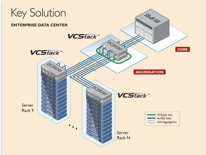
This network configuration enables servers and storage to communicate with low-latency high-speed connectivity. VCStack creates a single virtual unit out of two devices, ensuring no single point of failure.
